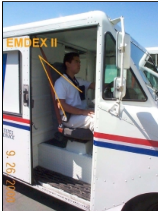
Photo 1: Meter Locations for the Driver
