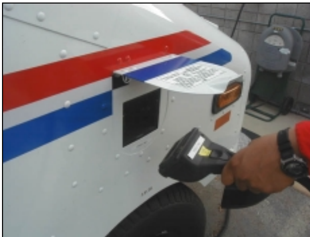
Figure 3-12 AVCON Charging Connector and Charge Port
