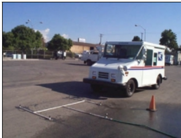
Figure 3-8 Water Test Setup
