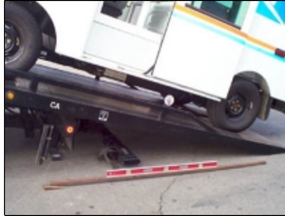
Figure 3-6 Gradeability Setup and Equipment at 25% Grade
