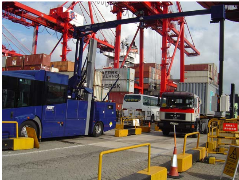
Figure 7. This picture demonstrates the ability of ICIS to screen transhipped cargo.
