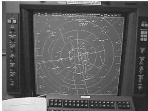
Figure 1: Standard Terminal Automation Replacement System Controller Workstation
