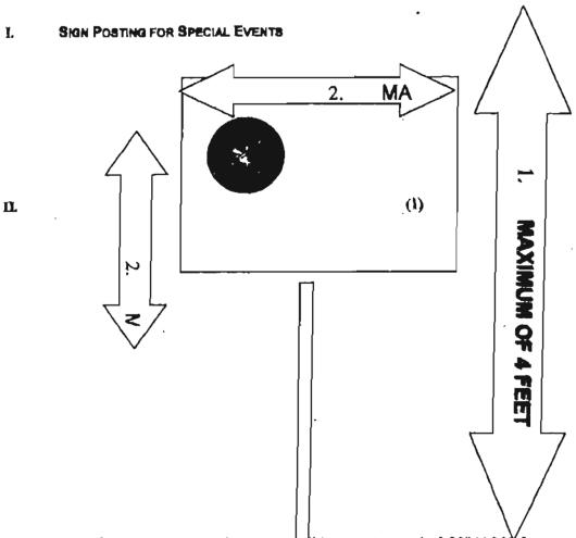
Signage indicating events or directions will be constructed of 20" X 30" foam core or poster board mounted on four (4) foat wooden or metal stakes using staples, noils or ties, (nylon or wire twist).
