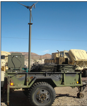
Figure 14: Transportable Hybrid Electric Power Stations (THEPS)
