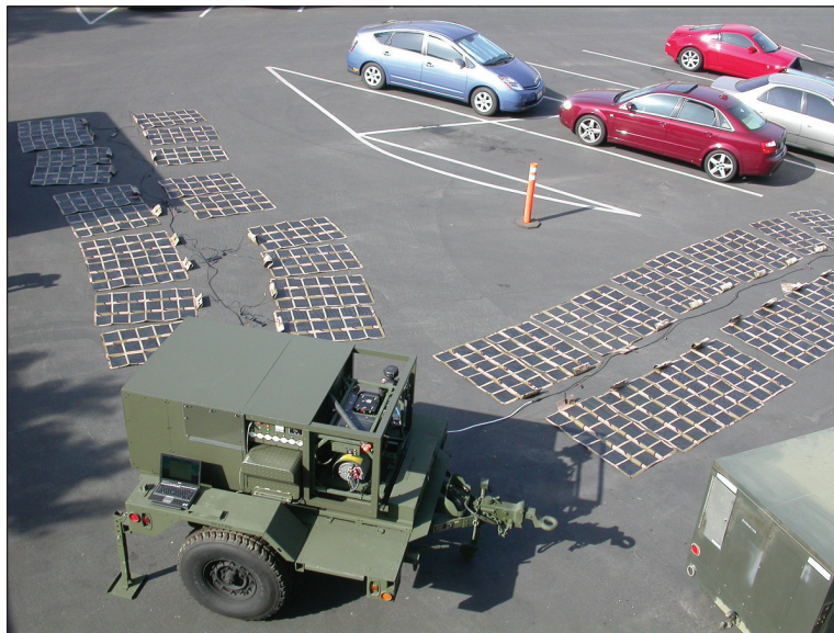
Figure 5: Deployable Renewable Energy Alternative Module Prototype
