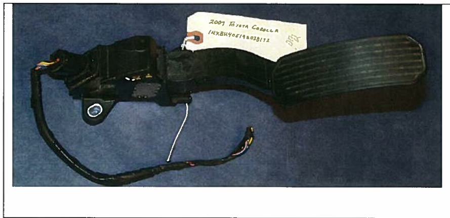
Figure 3. Accelerator pedal manufactured by CTS for an ETCS-i equipped 2009 Toyota Corolla
