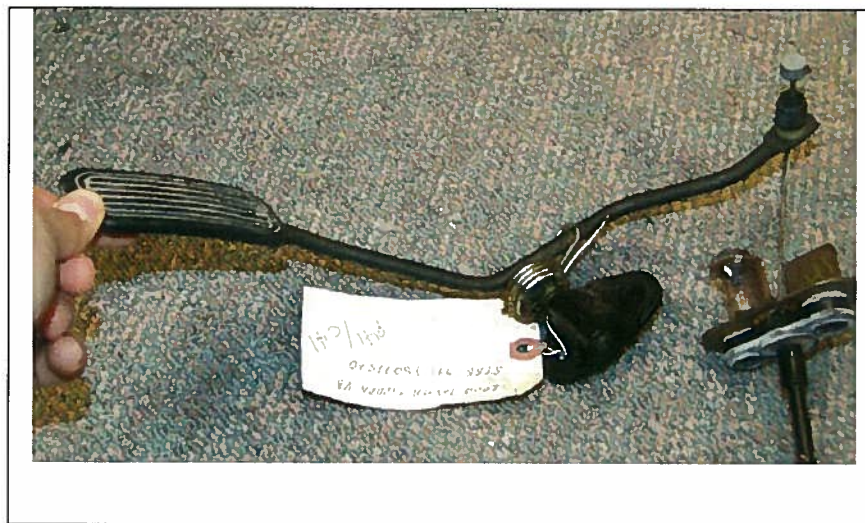
Figure 2. Pedal from a pre-ETCS-i Toyota Tundra
