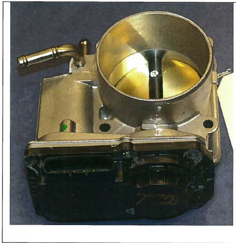
Figure 7. Throttle body from an ETCS-i vehicle
