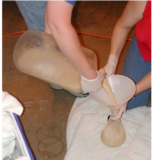
Pouring suspension of bacterial cells in preparation for pipe treatments within power plants. Advances in fermentation have allowed increasingly larger volumes of bacteria to be produced, thus allowing larger volumes of water to be treated in pipes.
