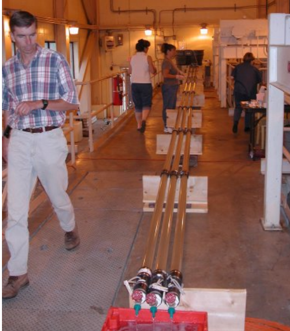
Very high zebra mussel kill (>95%) was consistently achieved in 6-hr treatments at 100 ppm inside a NYPA hydropower plant under flow-through conditions (3 replicate pipes 17 m in length were used in this trial). Experiments to date indicate that there should be no limit on the length of pipe that can be successfully treated.
