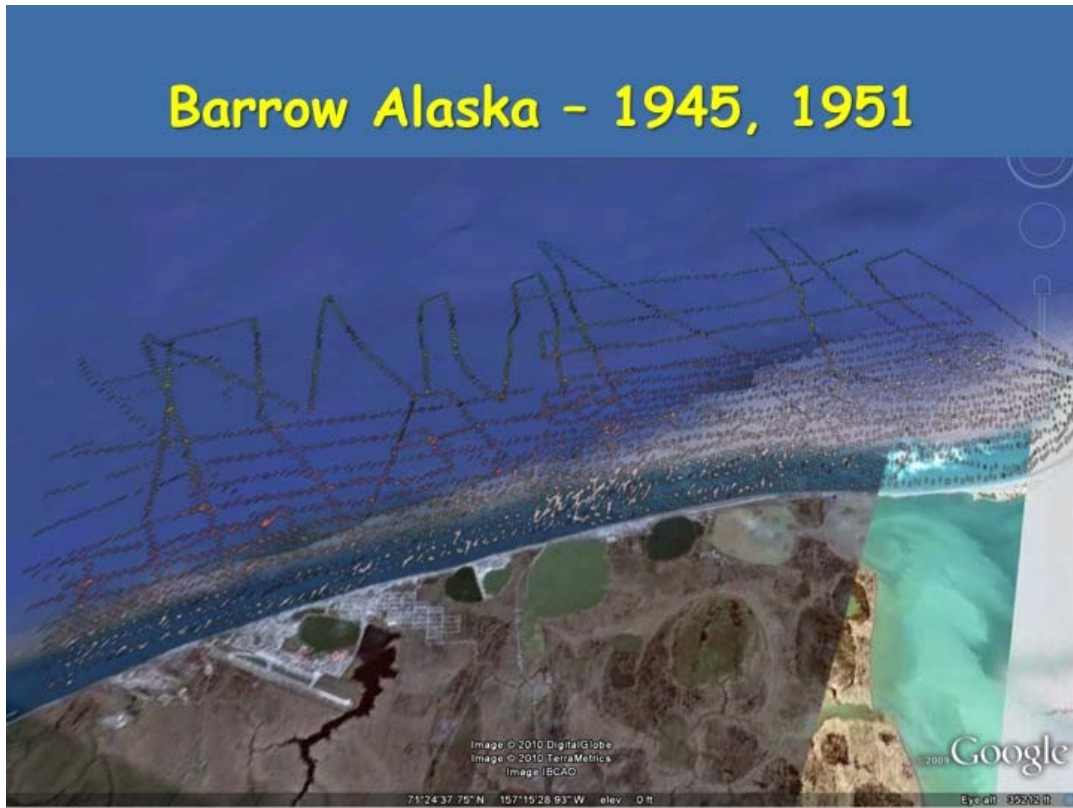
Figure 5. The total database of seafloor depth measurements for the area off Barrow Alaska. These data were collected in 1945 and 1951 and have not been updated since
