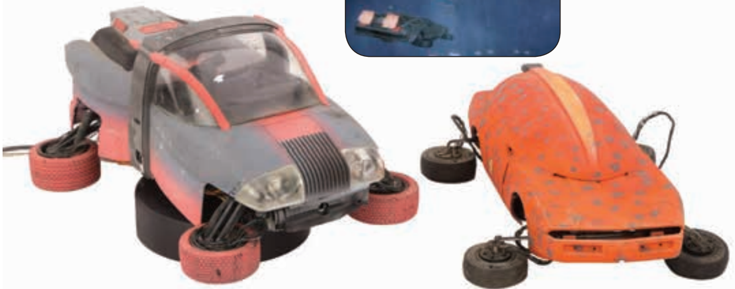
768. (2) SCREEN-USED FUTURE CARS FROM BACK TO THE FUTURE II. (Universal, 1989) (2) screen-used hover-car miniatures seen in Back to the Future II . These cars are on screen in the scene in which Doc Brown, Marty and Jennifer travel to the Hill Valley of 2015 and find themselves on a busy freeway in the sky. Both vehicles are constructed of resin, vacuum-formed plastic, rubber and are wired for illumination. (1) Red with gray polka dots, and modeled after a mid-'80s Corvette. Tail lights originally illuminated (along with headlights), but electronics are currently non-functioning. Shows light signs of use and wear. Measures approx. 11 x 4 x 3 1/2 in. (1) Gray-and-pink pickup truck with pink-painted wheels that originally illuminated on the underside, but are currently nonfunctioning. Measures approx. 11 x 5 x 8 in. Mounted to a custom display stand. Mild signs of production wear on both. $2,000 - $3,000
