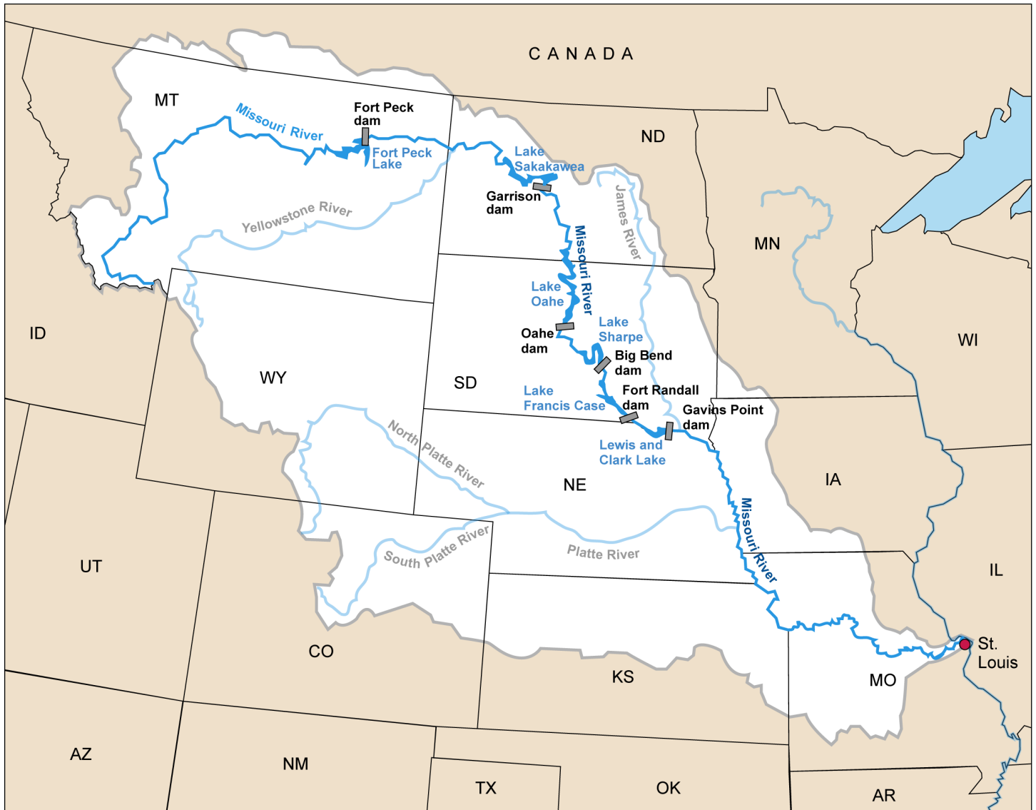
Figure 1: Missouri River Basin and the Six Mainstem Dams and Reservoirs
