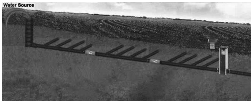
Schematic of sub-irrigation distribution of water into cropped field. Graphic courtesy of AgriDrain.
