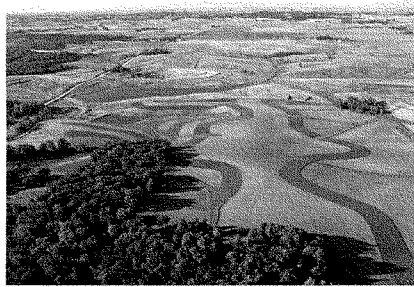
Figure 17. A small dam, terraces, buffer strips, and grass plantings are part of a conservation project to improve the quality of water entering Union Grove Lake in Tama County, Iowa. Photo credit: USDA-NRCS.
