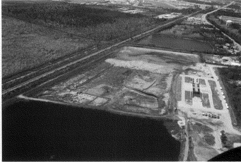
Figure 5: Chef Menteur Construction and Demolition Debris Landfill and previously operated municipal solid waste transfer station in New Orleans East. Hurricane debris can be seen being disposed of in the unlined disposal cell.
