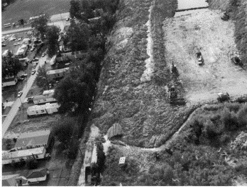
Figure 6: Photo showing Industrial Pipe Construction and Demolition Debris Landfill, Oakville, Plaquemines Parish. Industrial Pipe C & D Landfill disposes of hurricane debris in the unlined excavation and recycles white goods. The community of Oakville can be seen to the left, immediately adjacent to the Industrial Pipe Landfill to the right. A playground can be seen in the upper left corner with the graveyard just below the playground. Standing water can be seen (upper right corner) in the unlined pit that is being used to dispose of hurricane debris.
