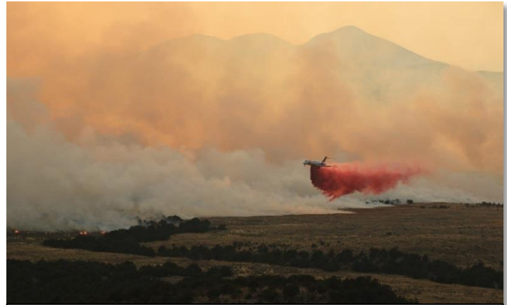
BLM Utah West Desert District, 2017 Sage Wild Fire – Air tanker drops retardant in a fuels treatment area. Fuels treatments and retardant are among the tools that aid suppression resources in attacking the fire and halting its progress.
