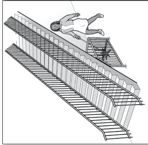
When the underside of a stair is open, it is a hazard to people who are blind or have low vision. Enclosing the area below the stair or installing a cane-detectable barrier helps the person to avoid the area.
