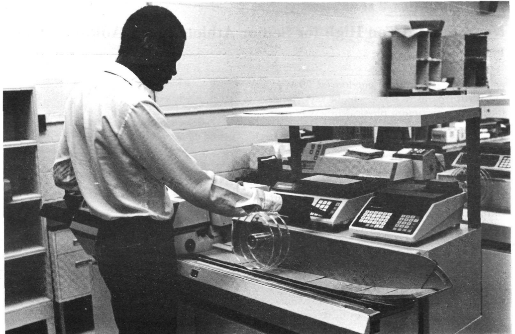
Terry Mundell, lead operator for the metered mailing machine system for the central mailroom in Bldg. 31, demonstrates how the metering works. The new system can process 207 letters per minute.
