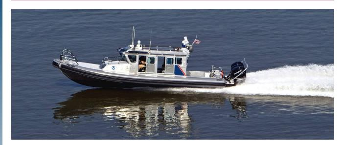
Marine interdiction agents with CBP's Air and Marine Operations use the 38-foot Secure Around Flotation Equipped (SAFE) Boat for the pursuit and boarding (inland and offshore) of vessels transiting in locations with extreme weather conditions.
