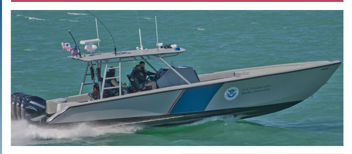
The Interim 40-foot SeaHunter Interceptor vessel provides maritime interdiction capabilities for CBP's Air and Marine Operations (AMO). These vessels fill operational gaps at marine units until the next-generation Coastal Interceptor Vessel is ready to deploy.
