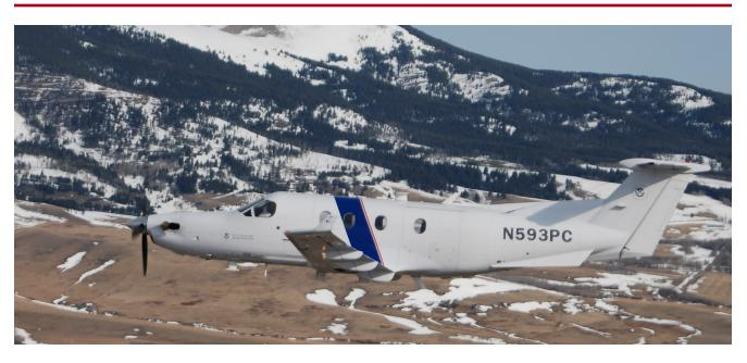
The PC-12 is a single-engine, turbo-prop, fixed-wing aircraft which combines slow-speed and high-speed capability, with a large payload capacity. These characteristics enable this aircraft to deploy rapidly and operate safely in remote areas.
