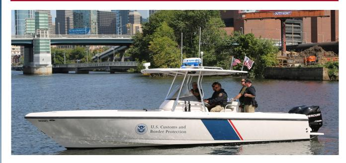
The 30-foot Intrepid coastal enforcement vessel provides a versatile maritime law enforcement capability. The hull design makes it ideal for enforcement operations in shallow, inland and near coastal waters.
