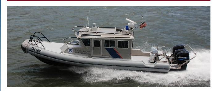
Marine interdiction agents with CBP's Air and Marine Operations (AMO) use the 33-foot Secure Around Flotation Equipped (SAFE) Boat for the pursuit and boarding (inland and offshore) of vessels transiting in locations with extreme weather conditions.
