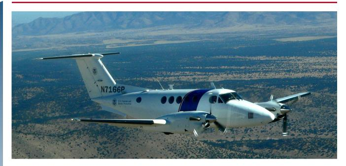
The Beechcraft King Air 200 and C-12C aircraft are medium-range, fixed-wing, twin turboprop aircraft used by U.S. Customs and Border Protection's Air and Marine Operations.
