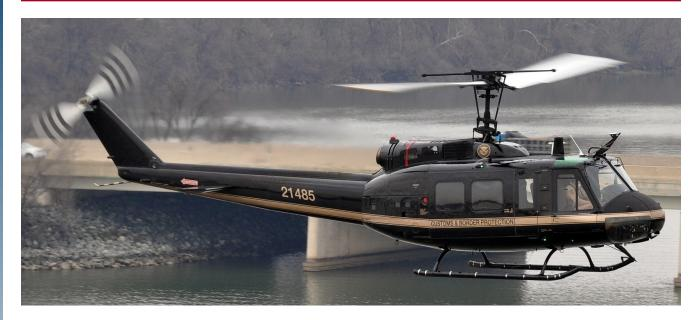
Bell UH-1H helicopters are short-range, turbinepowered helicopters which fly with a crew of two (pilot and copilot). The medium-lift capability of the UH-1H supports agents in high-altitude and hot environments, such as the desert in the Southwest Region, where pilots encounter extreme temperatures that may disrupt safe aircraft operation.
