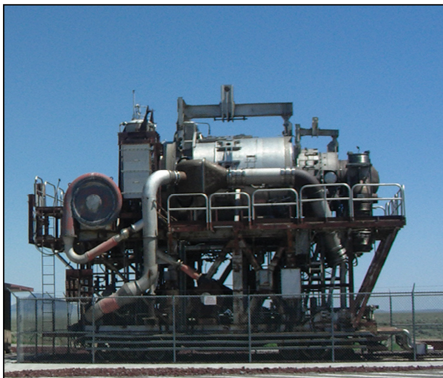
One of two experimental reactors for development of aircraft nuclear propulsion on display at the Idaho National Laboratory as of July 2009. Photo: Wtshymanski released to Creative Commons 3.0, December 2009.
