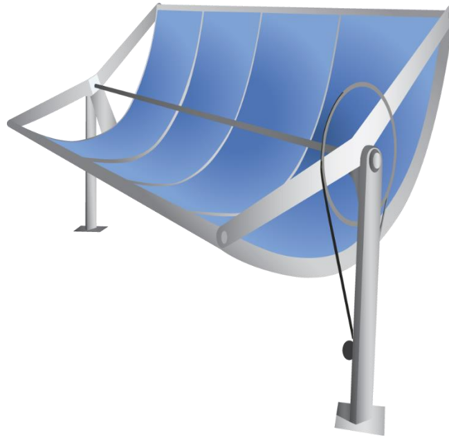
Figure 2: Typical Parabolic Trough Collector
