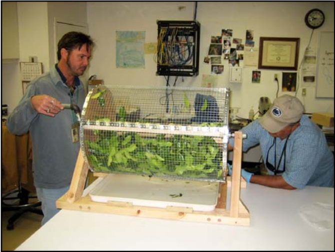
Figure 1. Raffle drum-type tumbler with catch tray.
