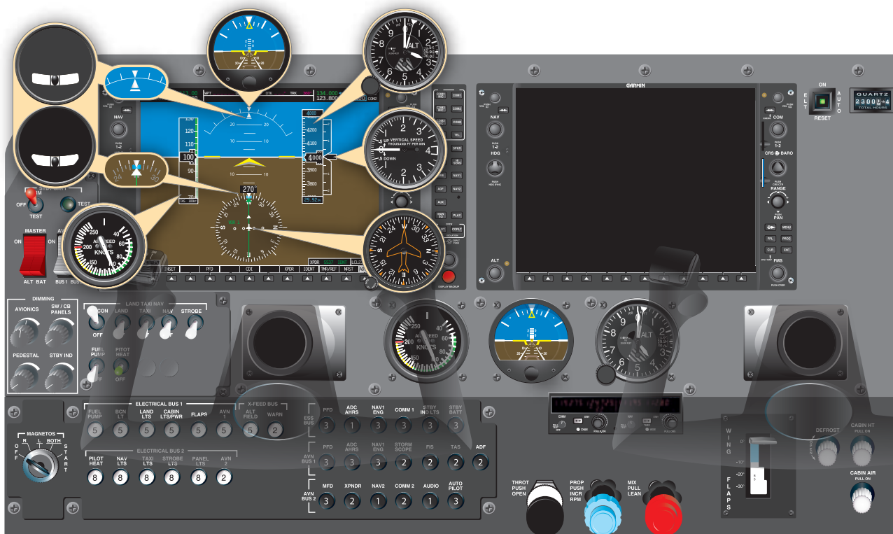
Figure 6-21. Primary flight display (PFD) and analog counterparts.
