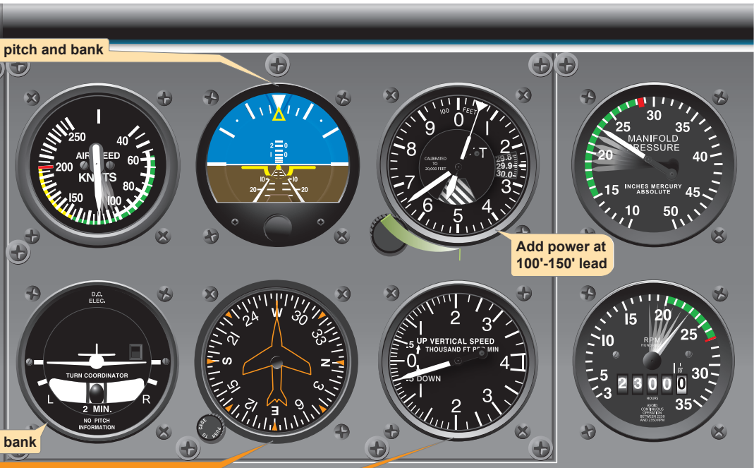
Figure 7-30. Constant airspeed descent, airspeed high—reduce power.
