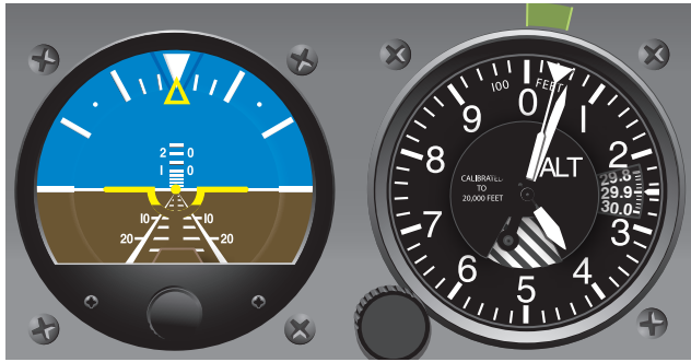
Figure 7-9. Altitude error, less than 100 feet.
