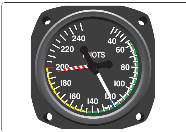
Figure 5-14. A maximum allowable ASI has a movable pointer that indicates the never-exceed speed, which changes with altitude to avoid the onset of transonic shock waves.
