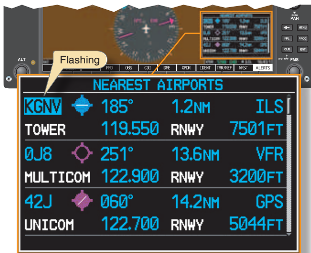
Figure 11-10. An enlargement of the box shown in the lower right of Figure 11-9. Note that KGNV would be flashing.
