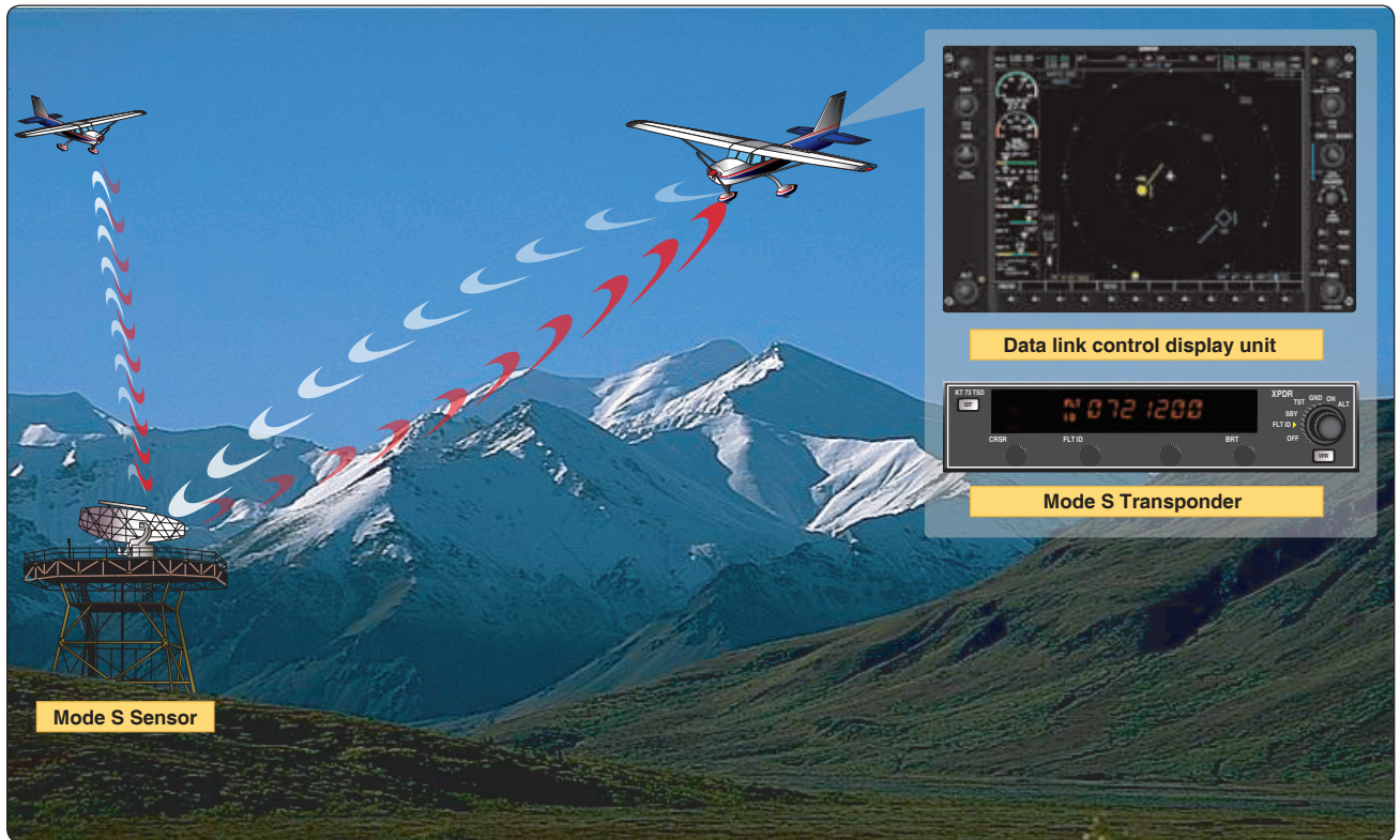
Figure 5-54. Concept of the traffic information system.
