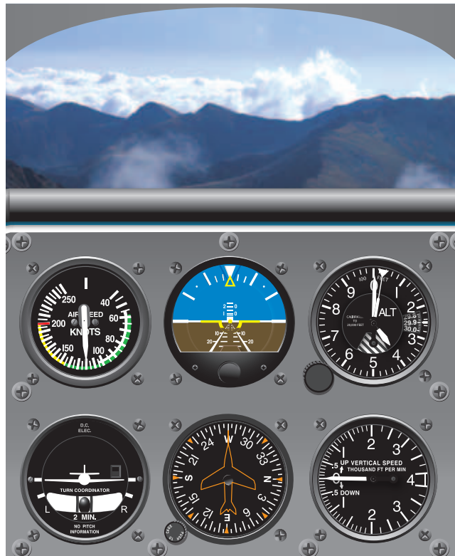
Figure 7-3. Pitch attitude and airspeed in level flight, normal cruise speed.
