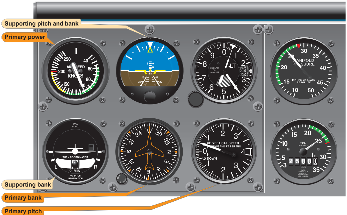
Figure 7-27. Stabilized climb at constant rate.
