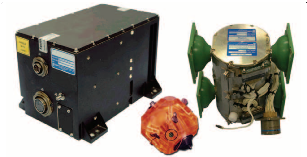
Figure 5-36. The Kearfott Attitude Heading Reference System (AHRS) on the left incorporates a Monolithic Ring Laser Gyro (MRLG) (center), which is housed in an Inertial Sensor Assembly (ISA) on the right.
