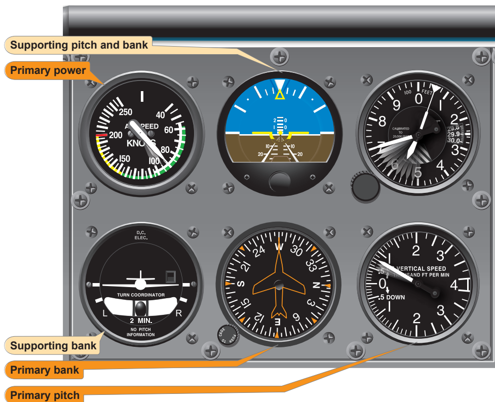
Figure 7-28. Airspeed low and vertical speed high—reduce pitch.
