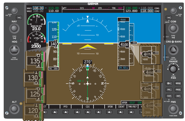
Figure 7-56. Figure shows both an increase in speed and altitude where pitch adjustment alone is insufficient. In this situation, a reduction of power is also necessary.
