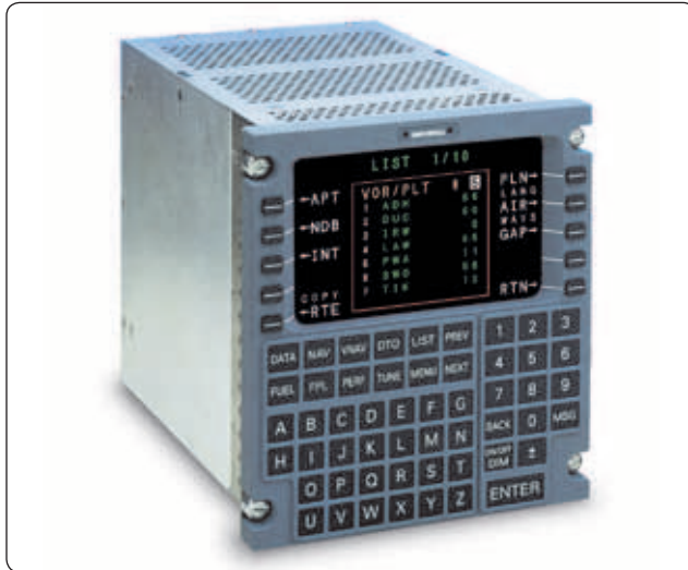
Figure 5-44. A Control Display Unit (CDU) used to control the flight management system (FMS).
