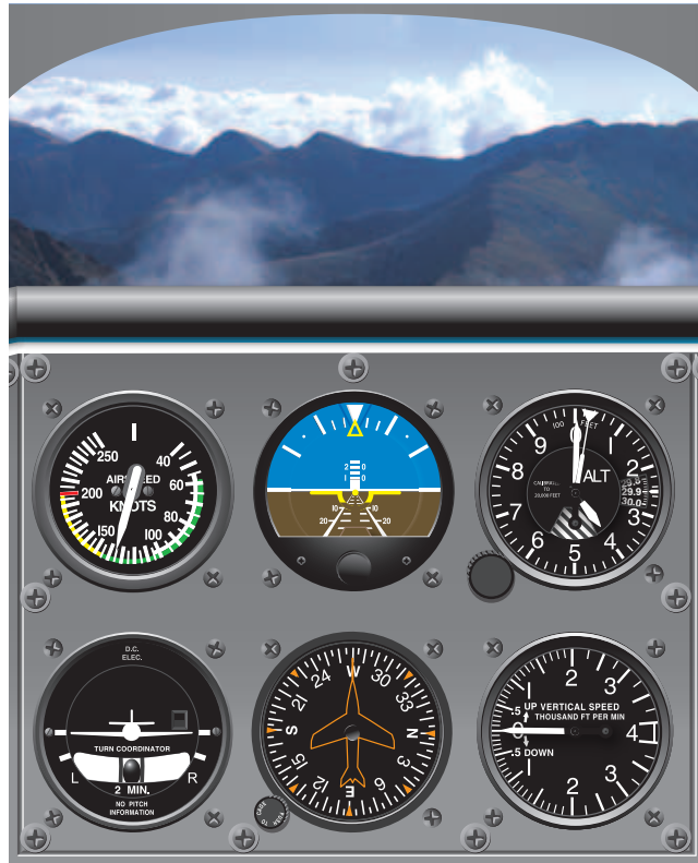
Figure 7-2. Pitch attitude and airspeed in level flight, fast cruise speed.
