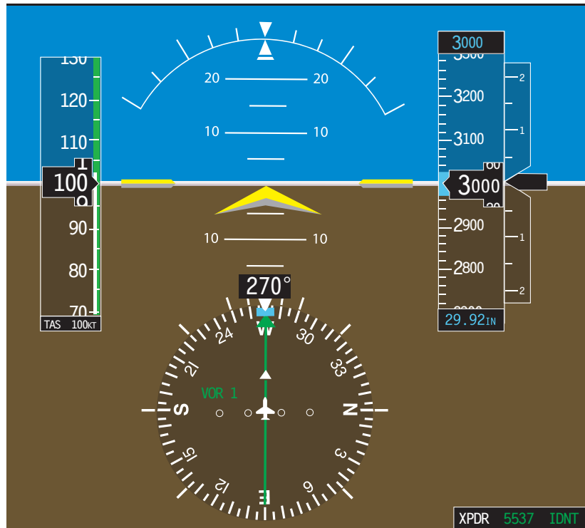
Figure 8-17. PFD indications during straight-and-level flight.
