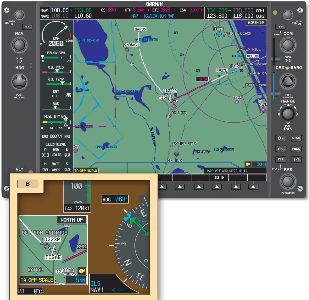
Figure 9-20. The same aircraft illustrated in Figure 9-19 shown on the ORM radial near TIGAE intersection turning inbound for the localizer.
