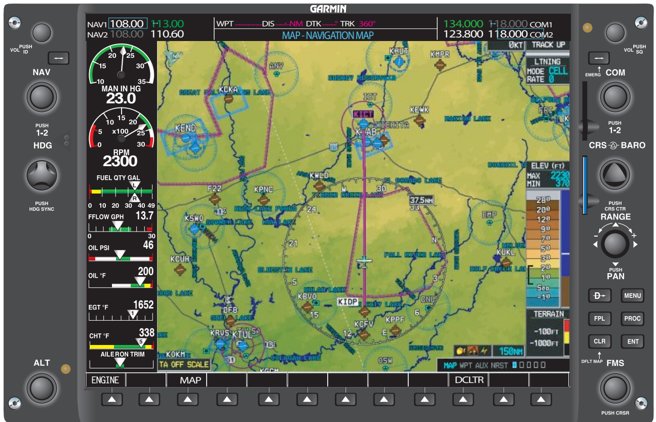
Figure 1-6. Moving map display.
