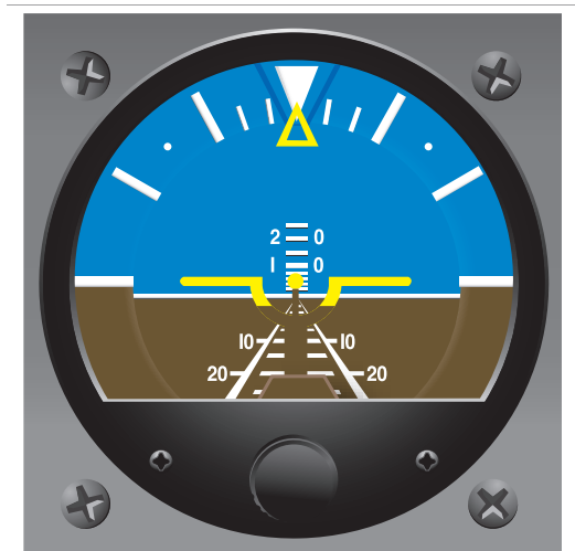
Figure 7-5. Pitch correction for level flight, one bar width.
