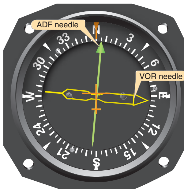
Figure 9-5. Radio magnetic indicator (RMI). Because the aircraft's magnetic heading (MH) is automatically changed, the relative bearing (RB), in this case 095°, indicates the magnetic bearing (095°) to the station (no wind conditions) and the MH that takes you there.
