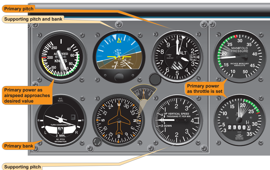
Figure 7-38. Change of airspeed during turn.
