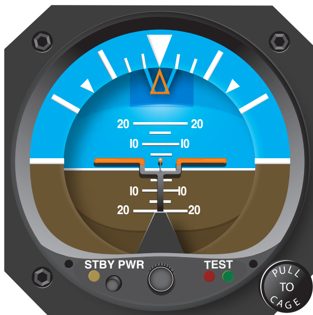
Figure 8-3. The initial pitch correction at normal cruise is one bar width or less.
