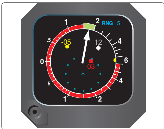
Figure 5-58. An example of a resolution advisory being provided to the pilot. In this case, the pilot is requested to climb, with 1,750 feet being the appropriate rate of ascent to avoid traffic conflict. This visual indication plus the audio warning provide the pilot with excellent traffic awareness that augments see-and-avoid practices.
