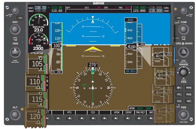
Figure 7-55. An aircraft decreasing in airspeed while gaining altitude. In this case, the pilot has decreased pitch.
