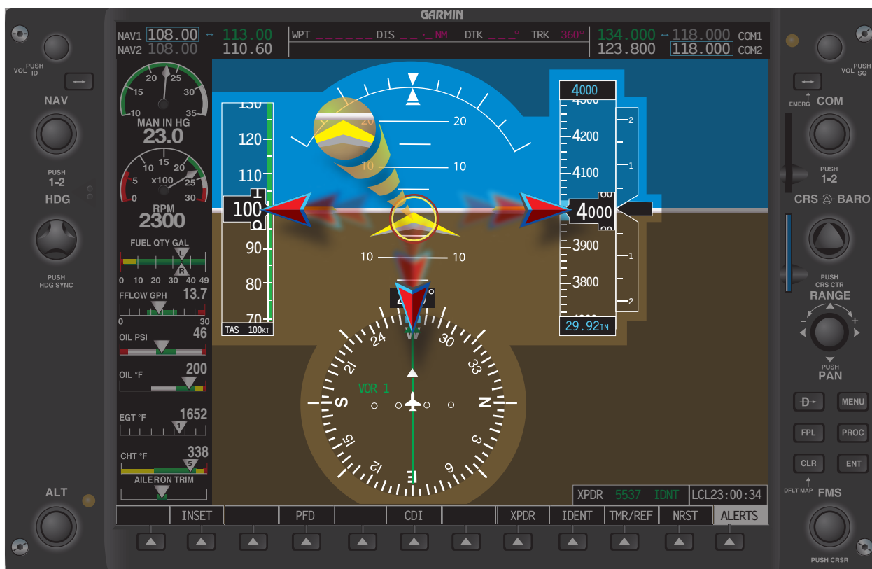
Figure 7-60. Cross-check supporting instruments.
