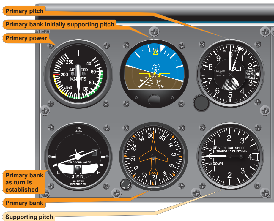
Figure 7-33. Standard rate turn, constant airspeed.
