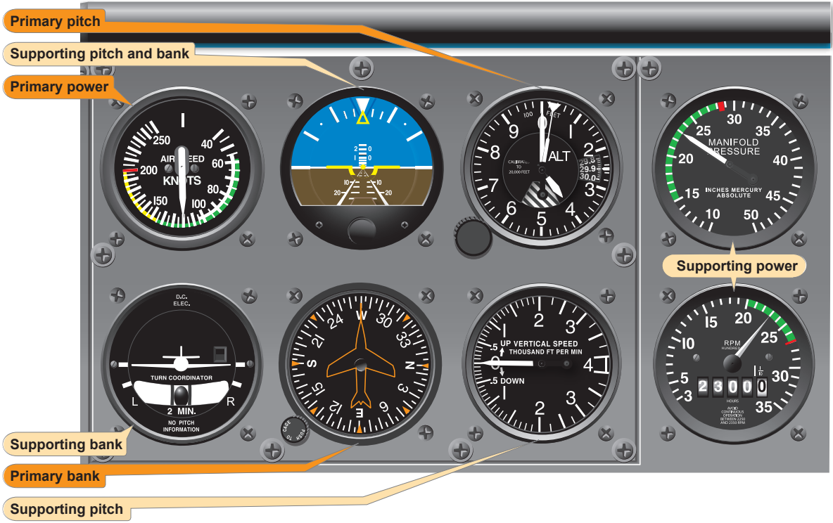
Figure 7-22. Straight-and-level flight (normal cruising speed).
