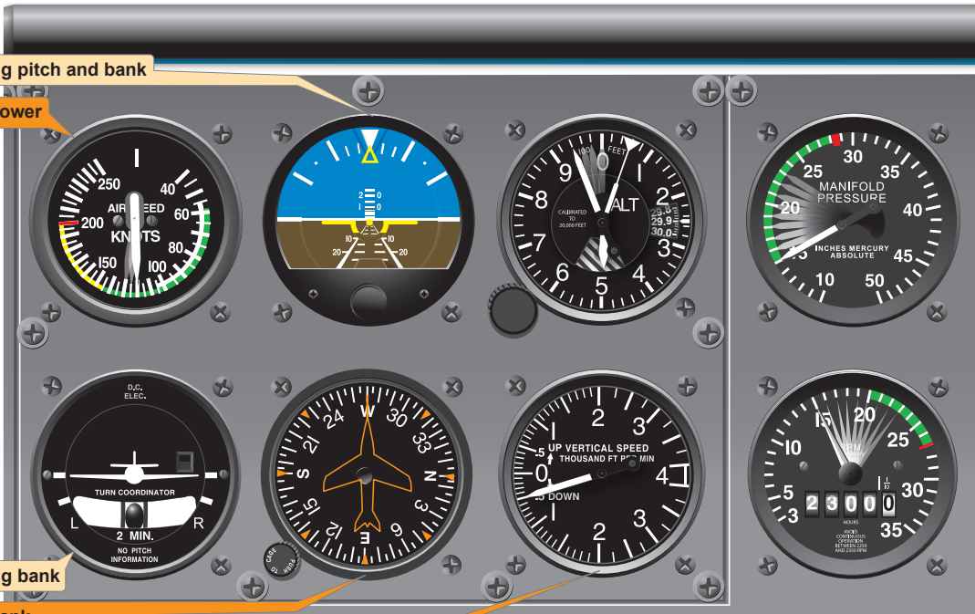
Figure 7-30. Constant airspeed descent, airspeed high—reduce power.
