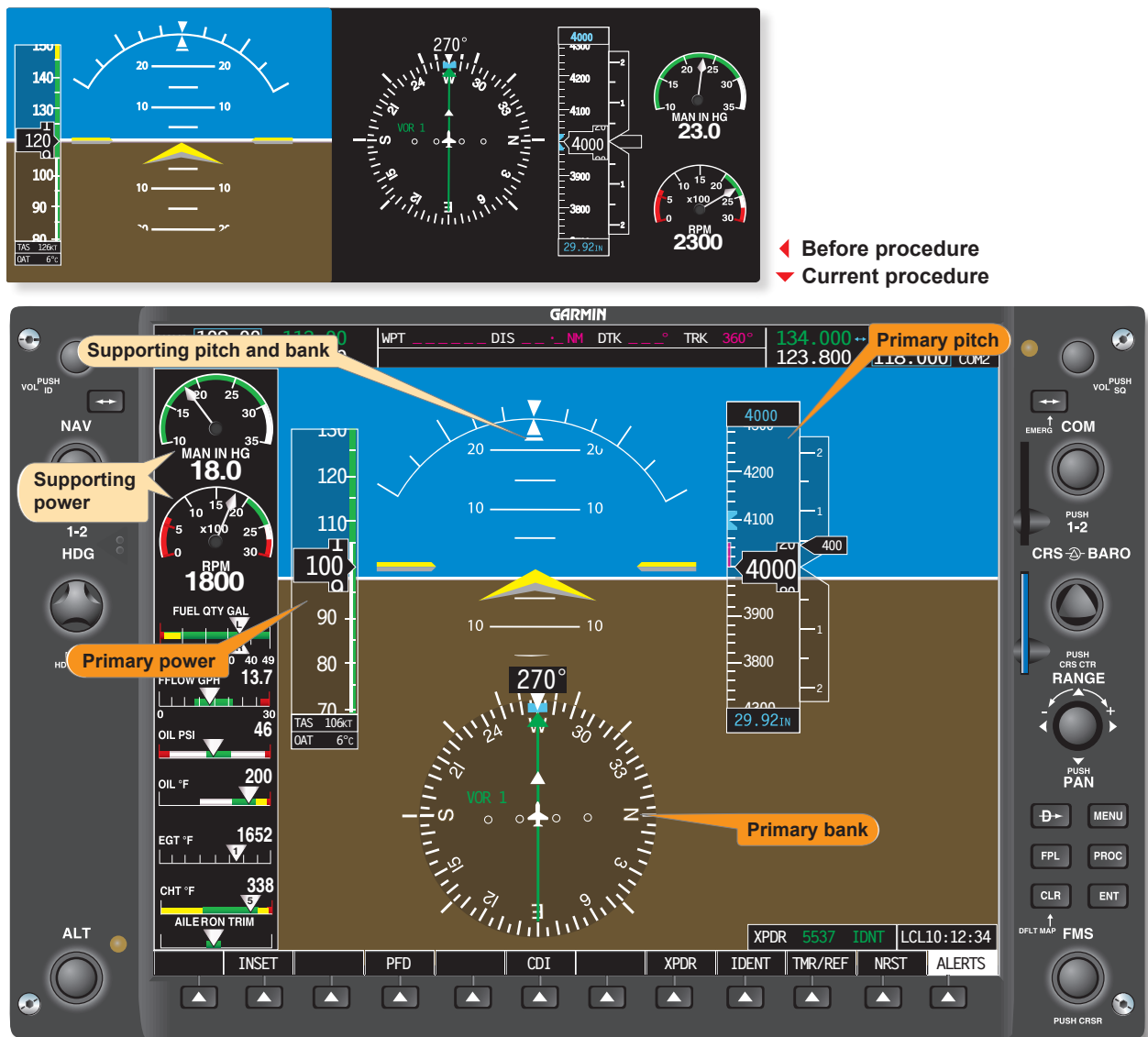
Figure 7-64. Constant airspeed climb from established airspeed.
