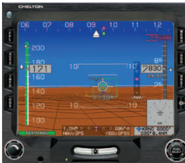
Figure 5-46. The benefits of realistic visualization imagery, as illustrated by Synthetic Vision manufactured by Chelton Flight Systems. The system provides the pilot a realistic, real-time, three-dimensional depiction of the aircraft and its relation to terrain around it.
