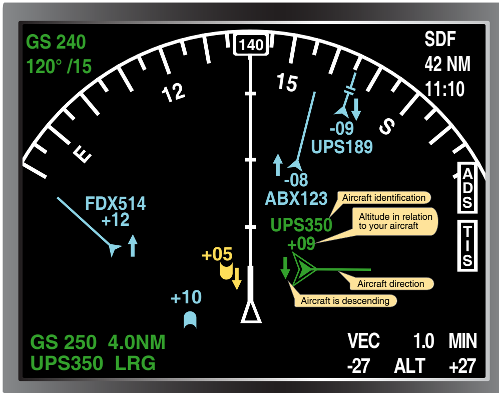
Figure 5-49. An aircraft equipped with ADS will receive identification, altitude in hundreds of feet (above or below using + or-), direction of the traffic, and aircraft descent or climb using an up or down arrow. The yellow target is an illustration of how a non-ADS equipped aircraft would appear on an ADS-equipped aircraft's display.
