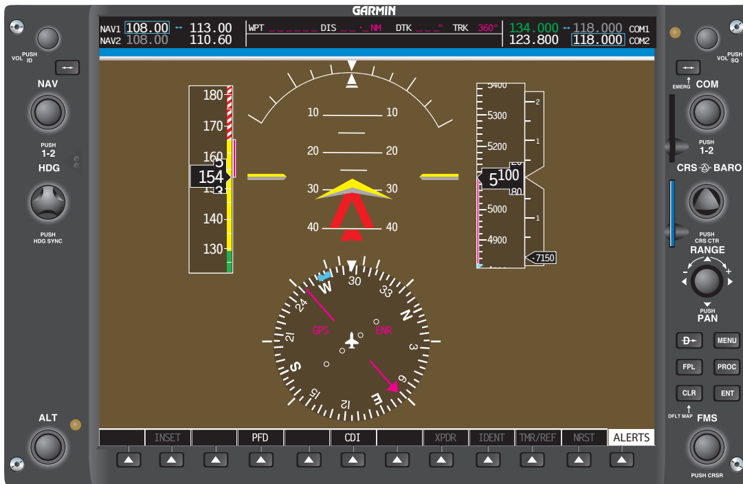
Figure 7-70. Horizon line starts moving upward at 27°. Note that the blue sky remains visible at 17° nose-down.
