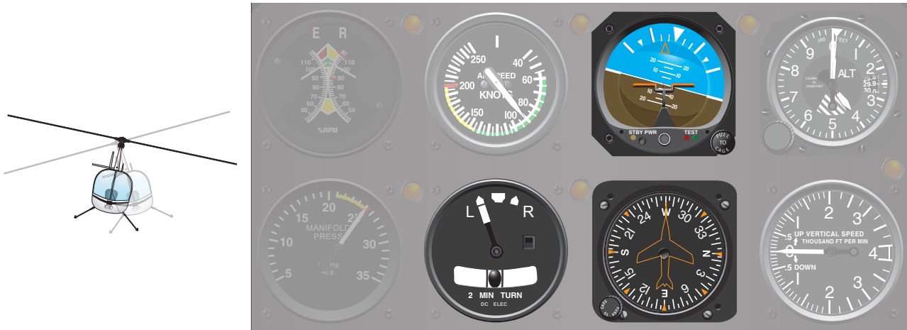
Figure 8-4. The flight instruments used for bank control are the attitude, heading, and turn indicators.
