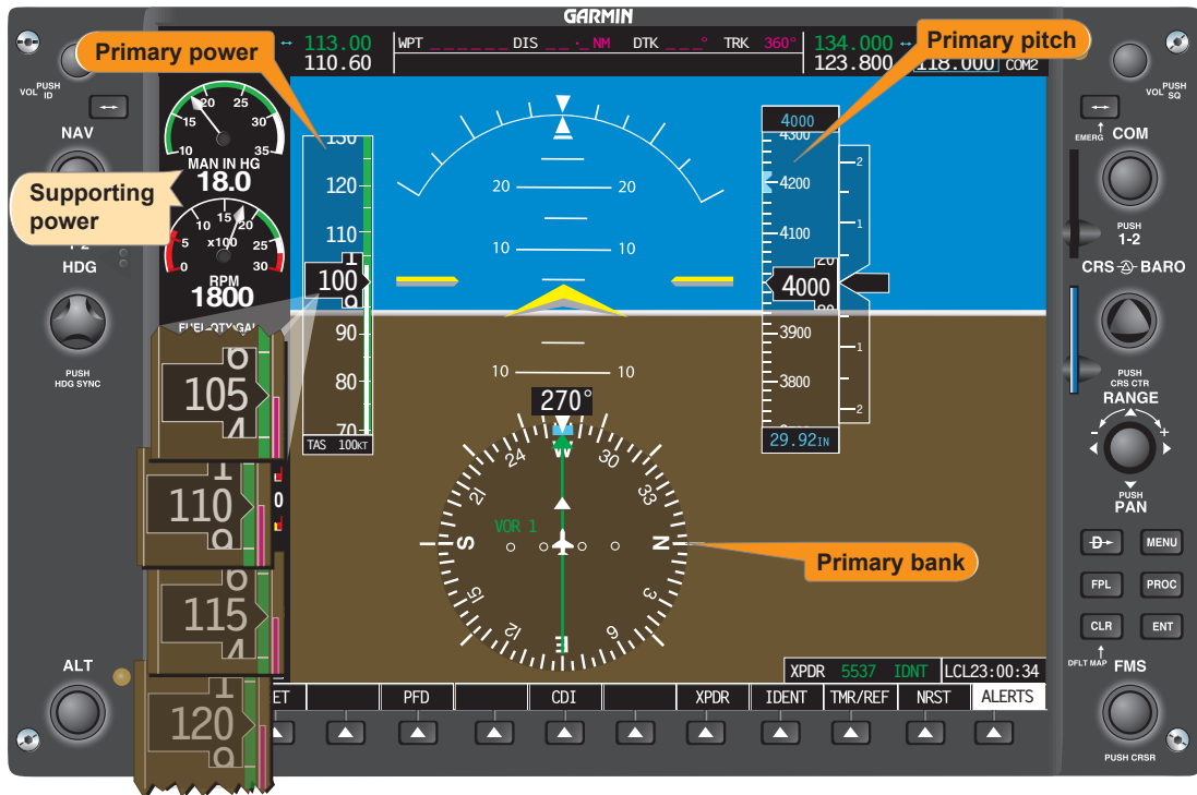
Figure 7-59. Straight-and-level flight (reduced airspeed stabilized).
