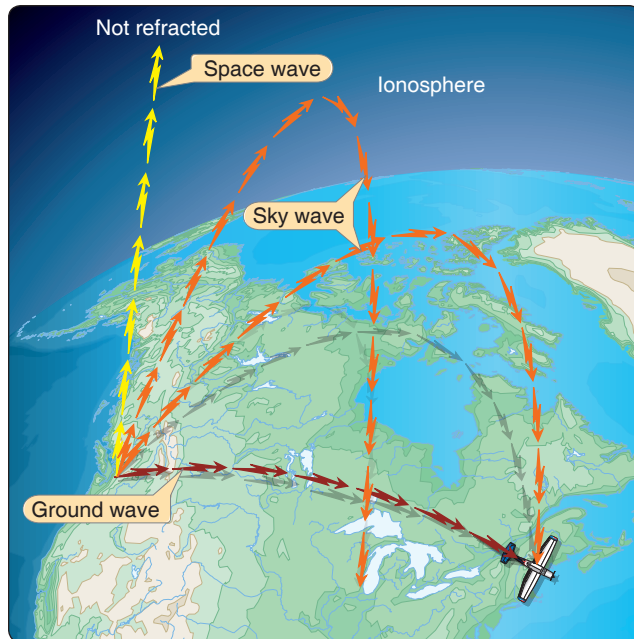
Figure 9-1. Ground, space, and sky wave propagation.
