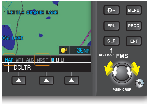
Figure 11-14. Page groups. As the FMS outer knob is rotated, the current page group is indicated by highlighting the specific group indicator. Notice that the MAP page group is highlighted.
