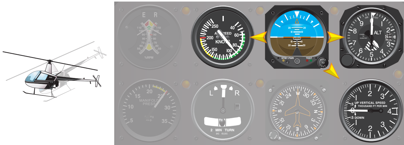
Figure 8-2. The flight instruments for pitch control are the airspeed indicator, attitude indicator, altimeter, and vertical speed indicator.
