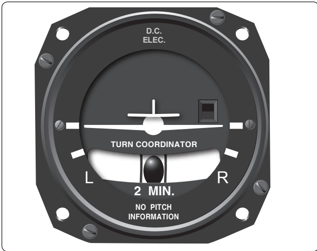
Figure 5-35. A turn coordinator senses rotation about both roll and yaw axes.
