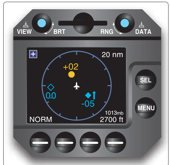
Figure 5-56. A Skywatch System.
