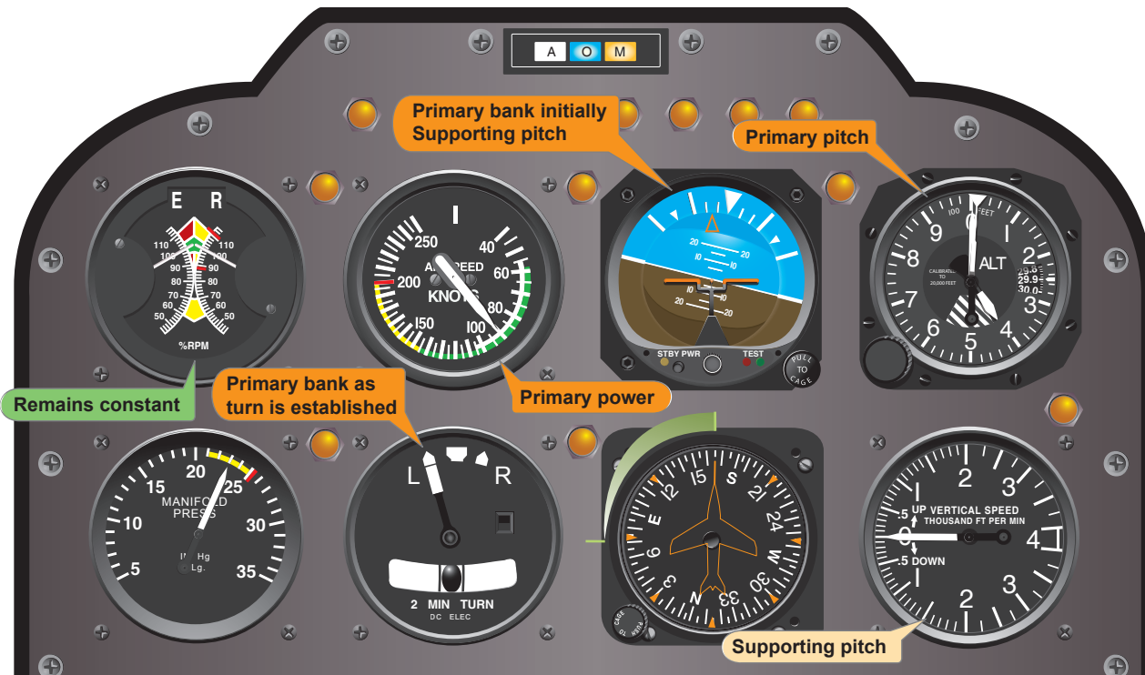
Figure 8-14. Flight instrument indications in a standard-rate turn to the left.
