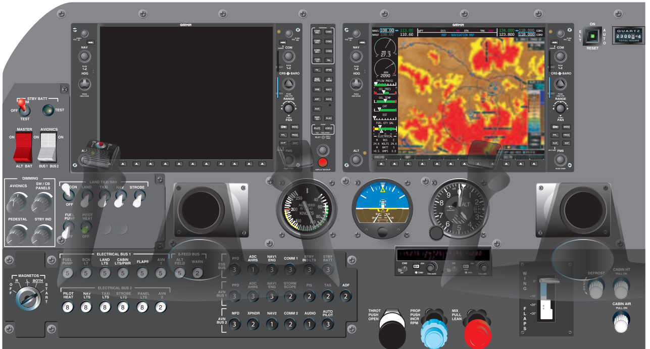
Figure 6-22. Multifunction display (MFD).
