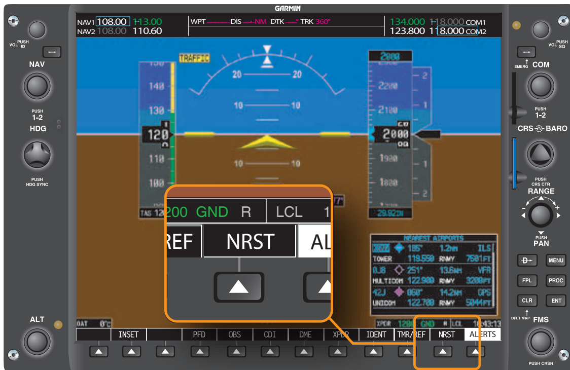
Figure 11-9. The default soft key menu that is displayed on the PFD contains a “NRST” (Nearest Airport) soft key. Pressing this soft key opens a text box that displays the nearest 25 airports.
