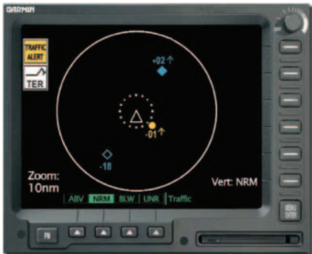
Figure 5-57. Alert System by Avidyne (Ryan).
