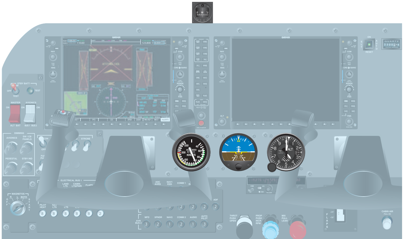
Figure 11-7. Emergency instrumentation available to the pilot on electronic flight instrumented aircraft.
