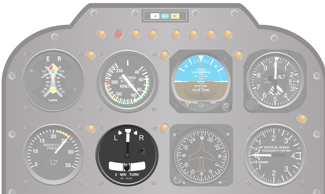
Figure 8-6. Coordinated flight is indicated by centering of the ball.
