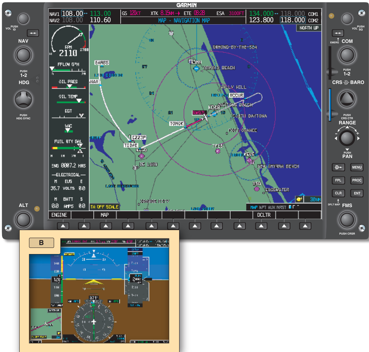
Figure 9-21. Aircraft is illustrated inbound on the localizer course.
