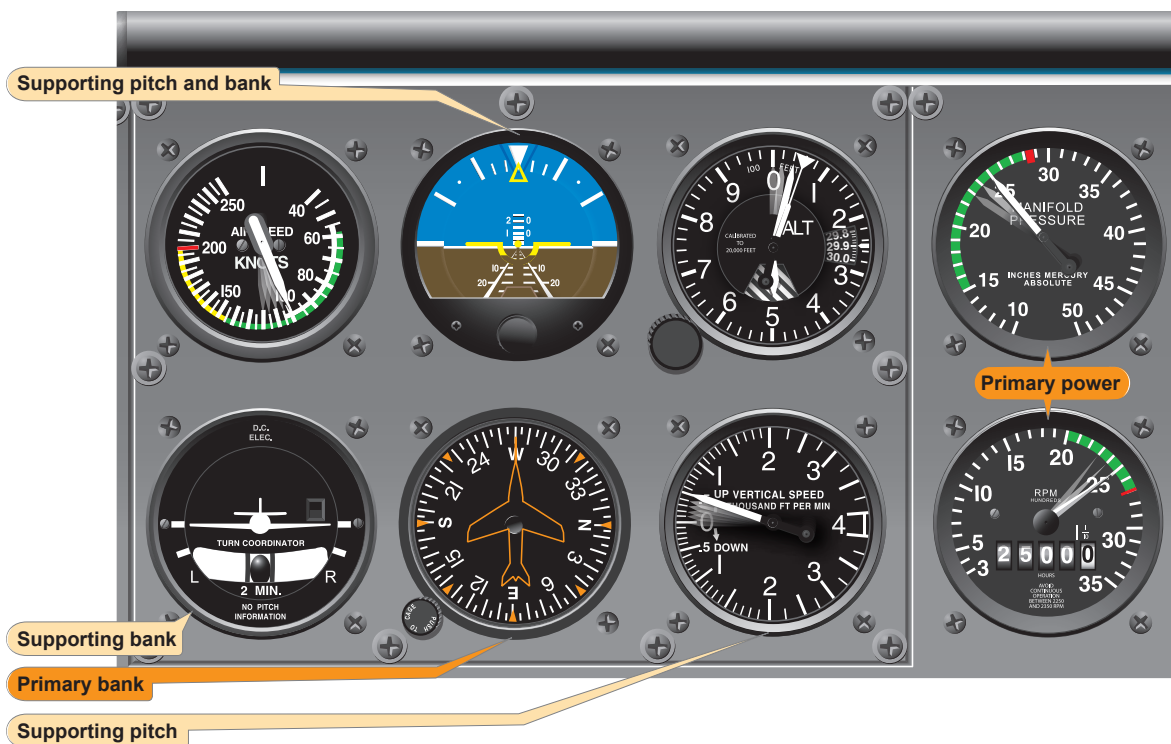
Figure 7-25. Climb entry for constant airspeed climb.
