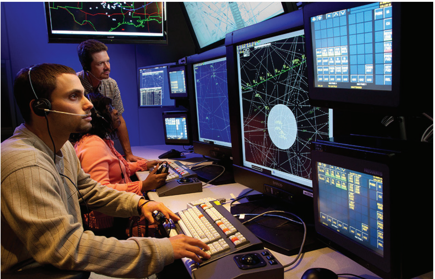
ERAM is the new FAA computer system used to control high altitude air traffic.
