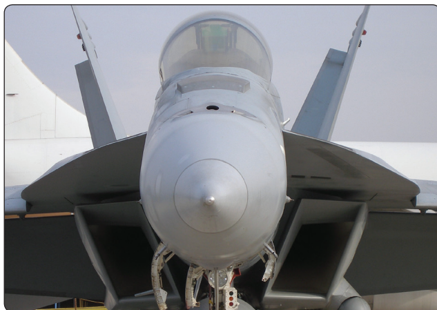
Figure 3-25. An example of a divided-entrance duct.
