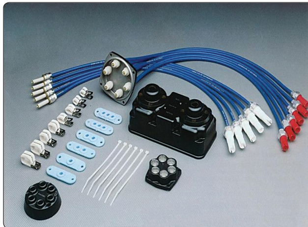
Figure 4-11. A high-tension ignition harness.
