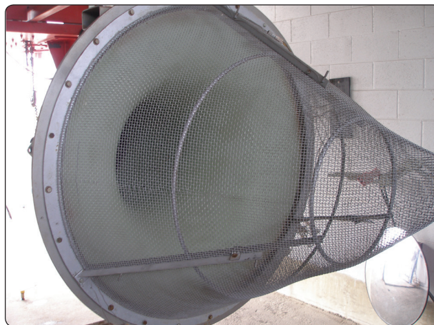
Figure 3-30. A bellmouth inlet used during system tests.
