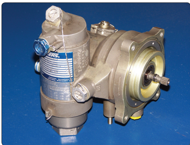
Figure 2-50. Fuel pump and filter.
