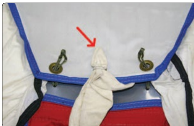
Figure 2-11. Square reserve hesitator loop configuration.
