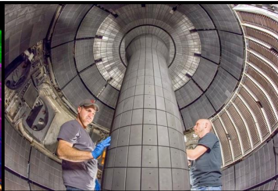
New central solenoid magnet inside NSTX-U upgrade
