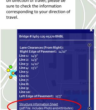
Bridge #:1465-125-05270 BNBL I-465 NB bridge over I-69, SR 37 0 Travel Direction: Northeast Minmum Clearance: 14'9" (14.78') Horizontal Clearance: 79'1" (79.1') Lane Clearances (From Pight): Right Edge of Pavement: 14'10" Line 1: 14'9" Line 2: 14'9" Line 3: 14'11" Line 4: 15'2" Line 5: Line 6: Line 7: Line 8: Line 9: ٥ Line 10: Zoom to
