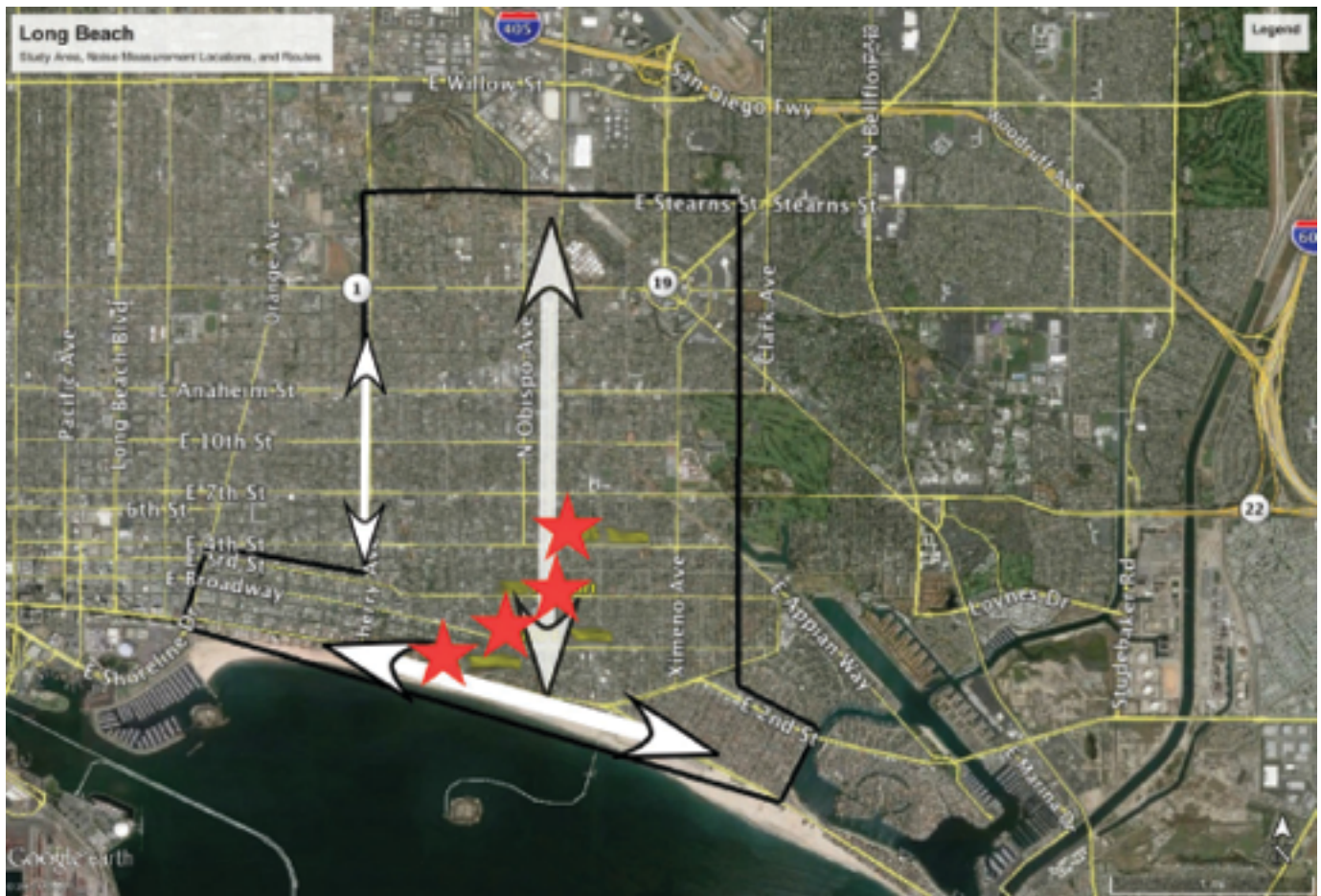
Figure 4-1. Helicopter routes (white double-ended arrows) and noise measurement sites (red stars) in Long Beach study area.
