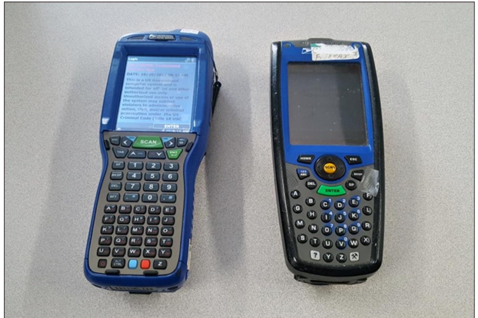
Figure 4: Devices Used by U.S. Postal Service to Scan Barcodes—Mobile Delivery Device (left) and Intelligent Mail Device (right)
