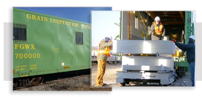
The Master Scale Depot is used to calibrate railroad test weight cars that are used to calibrate railroad track scales throughout the country. FGIS also has two specialized test weight cars that are used primarily to test and calibrate commercial railroad track scales.
