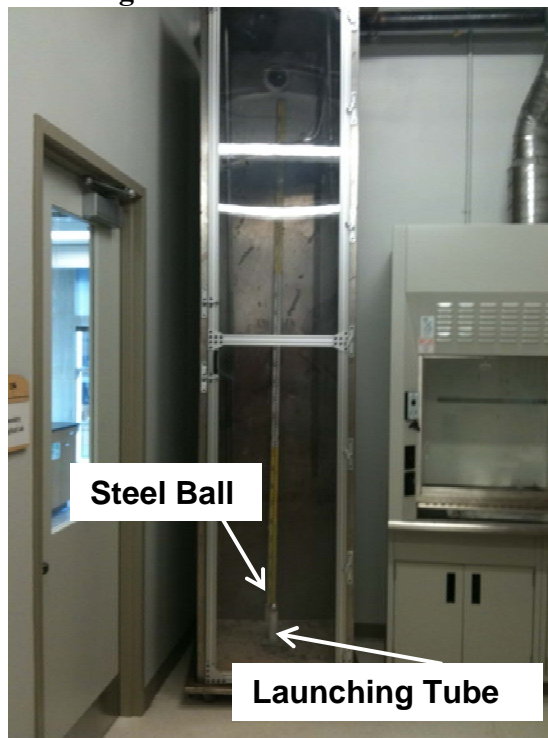
Figure 5: Metal “Blast Box”
