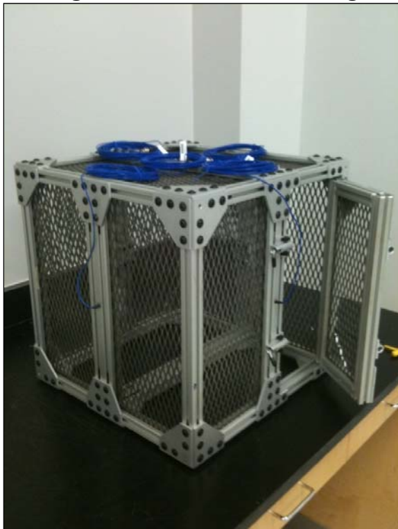
Figure 7: Constructed Blast Cage
