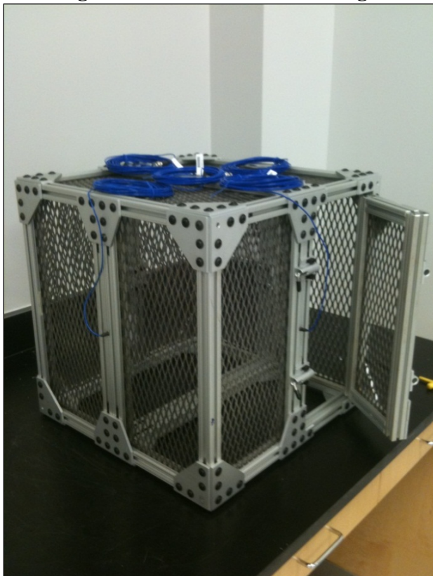
Figure 2: Constructed Blast Cage
