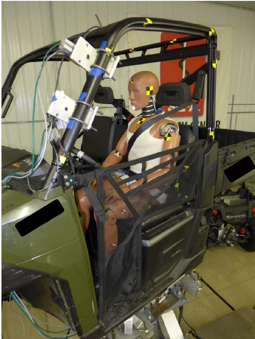
Figure B-5: Vehicle L15 on the Roll Simulator - Standard Tests
