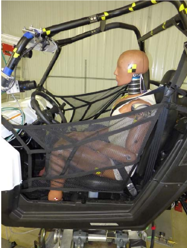
Figure 18: Vehicle M15 on the Roll Simulator - Additional Tests, No Bar, Hybrid III 50 th Percentile Male
