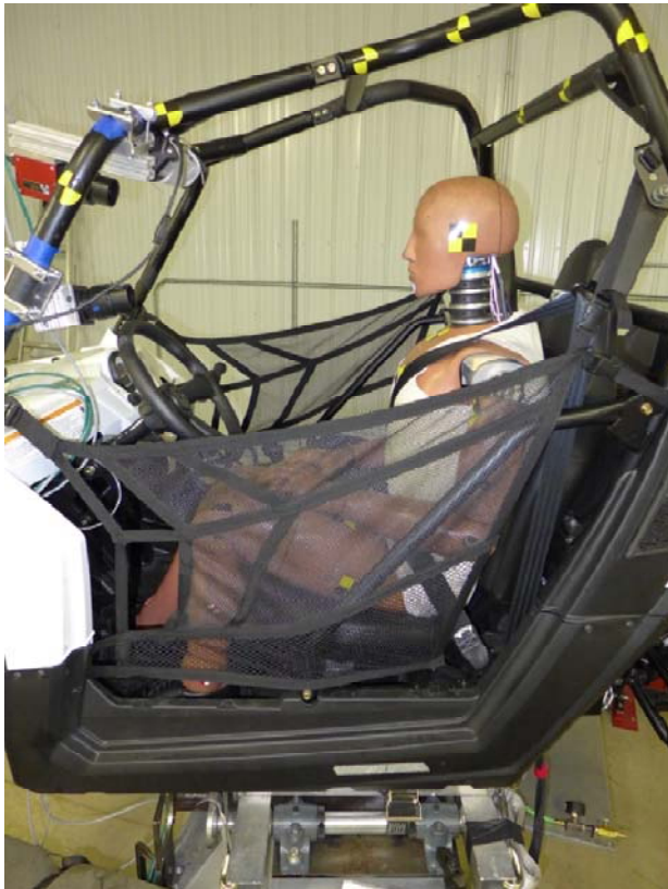
Figure 16: Vehicle M15 on the Roll Simulator - Additional Tests, Full Restraint System, Hybrid III 50 th Percentile Male
