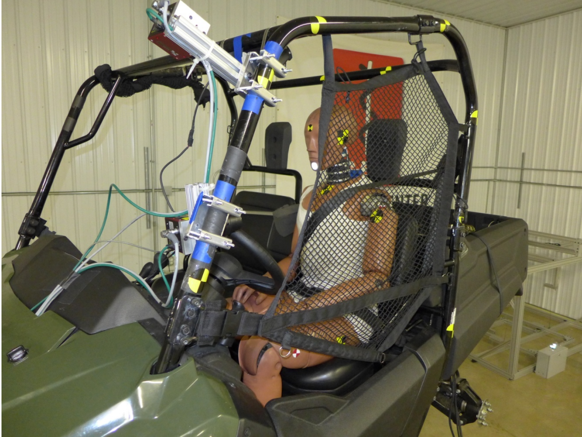
Figure B-4: Vehicle J15 on the Roll Simulator - Standard Tests
