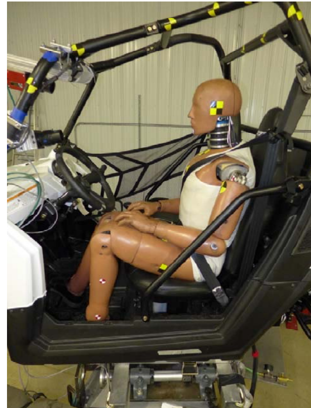
Figure 17: Vehicle M15 on the Roll Simulator - Additional Tests, No Net, Hybrid III 50 th Percentile Male
