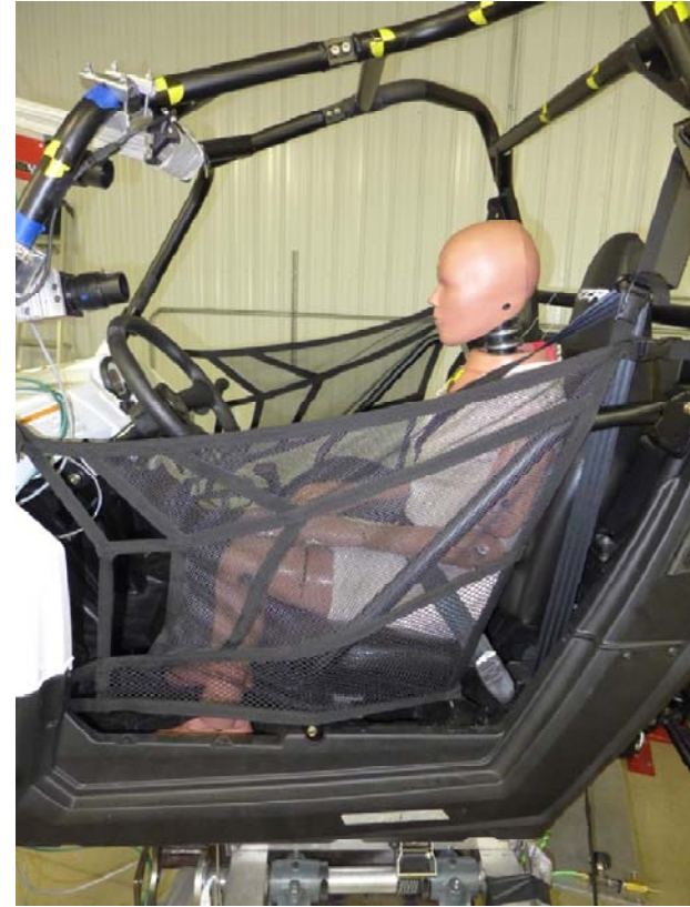
Figure 21: Vehicle M15 on the Roll Simulator - Additional Tests, Full Restraint System, 5 th Percentile Male
