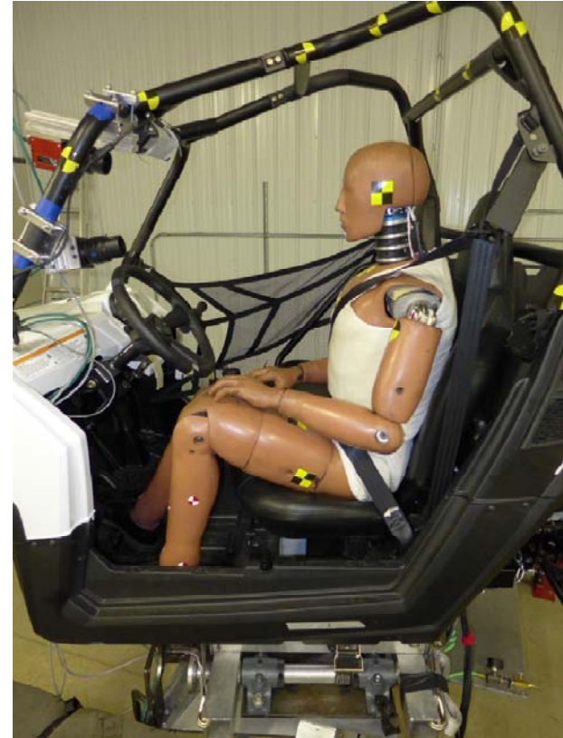
Figure 19: Vehicle M15 on the Roll Simulator - Additional Tests, No Net + No Bar, Hybrid III 50 th Percentile Male
