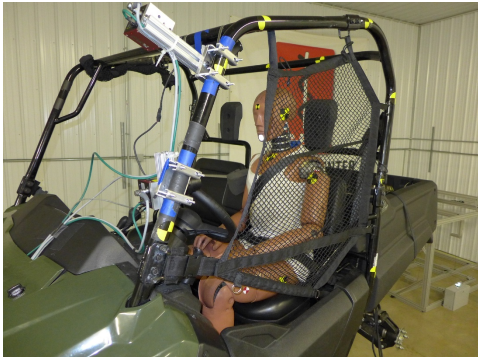
Figure 6: Vehicle J15 on the Roll Simulator - Standard Tests
