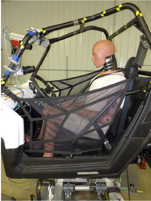
Figure 20: Vehicle M15 on the Roll Simulator - Additional Tests, Full Restraint System, 95 th Percentile Male
