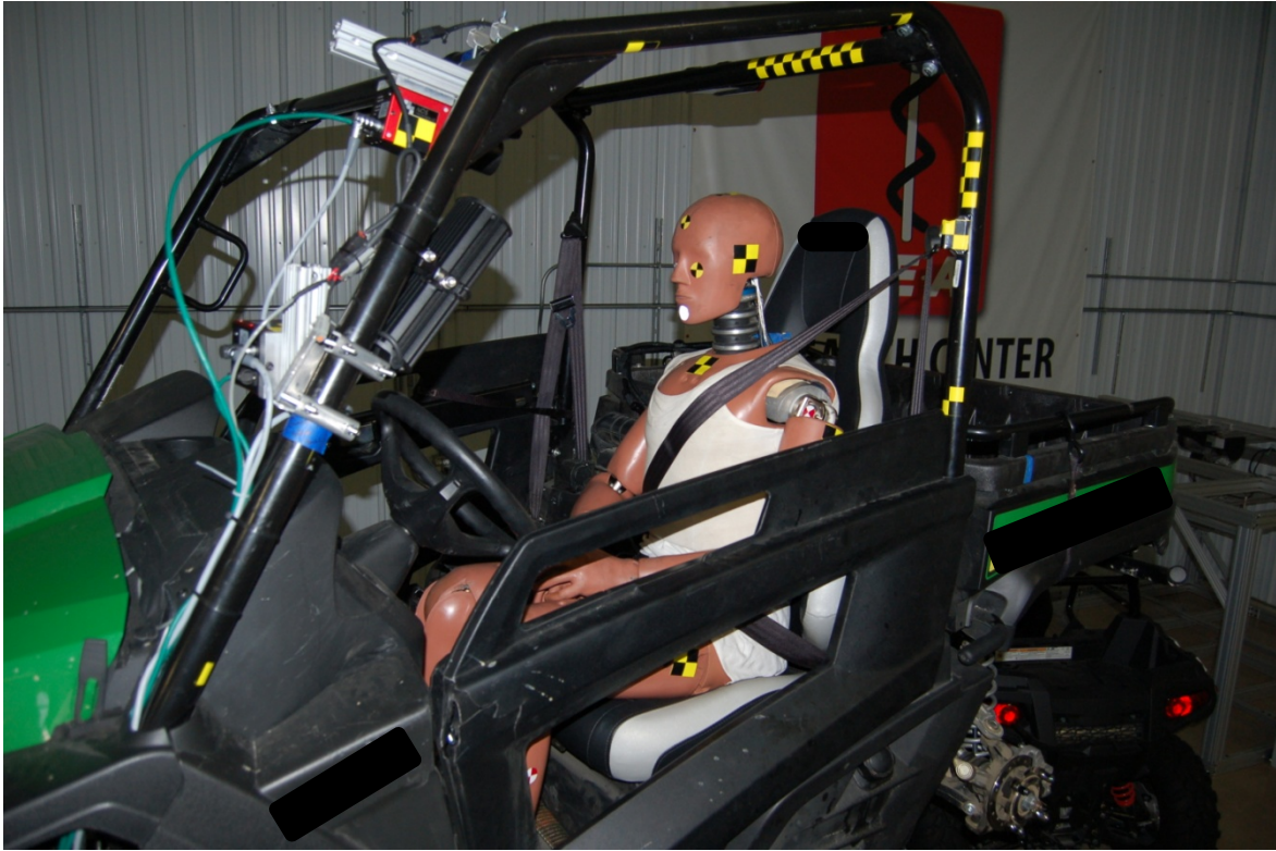
Figure B-3: Vehicle H15 on the Roll Simulator - Standard Tests
