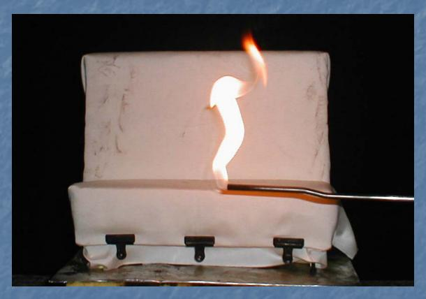
Nominal 240 mm flame, 70 sec. exposure, standard rayon cover fabric, standard polyurethane foam substrate
