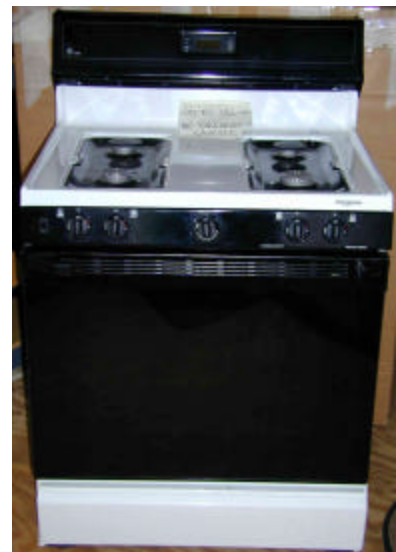
Figure 4. Gas Range used in Delayed-Ignition Tests
