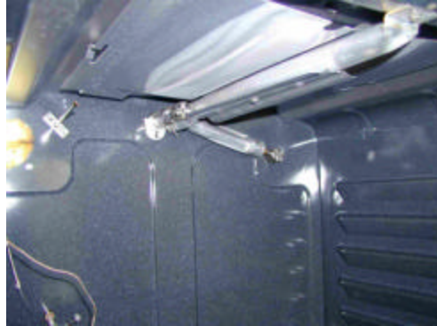
Figure 17. View inside Suction-Draft Range Showing Broiler Igniter and Burner
