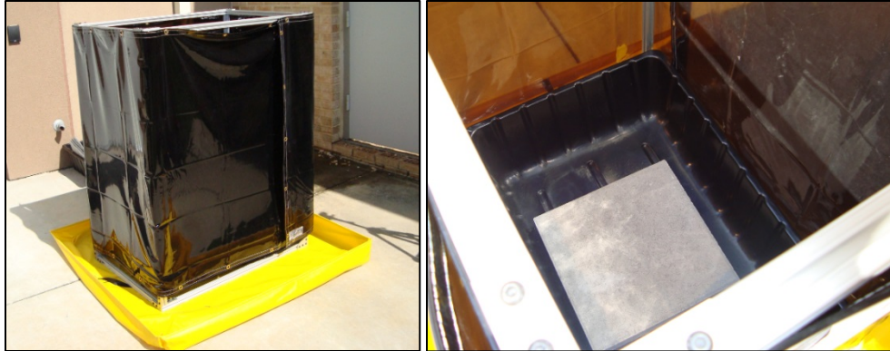
Figure 21 – Left: Protective Aluminum Frame Shield with Plastic Panels to Minimize Any Antifreeze Splashes Due to Drop Impact Testing; Right – Top View showing the Concrete Slab (Striking Surface)
