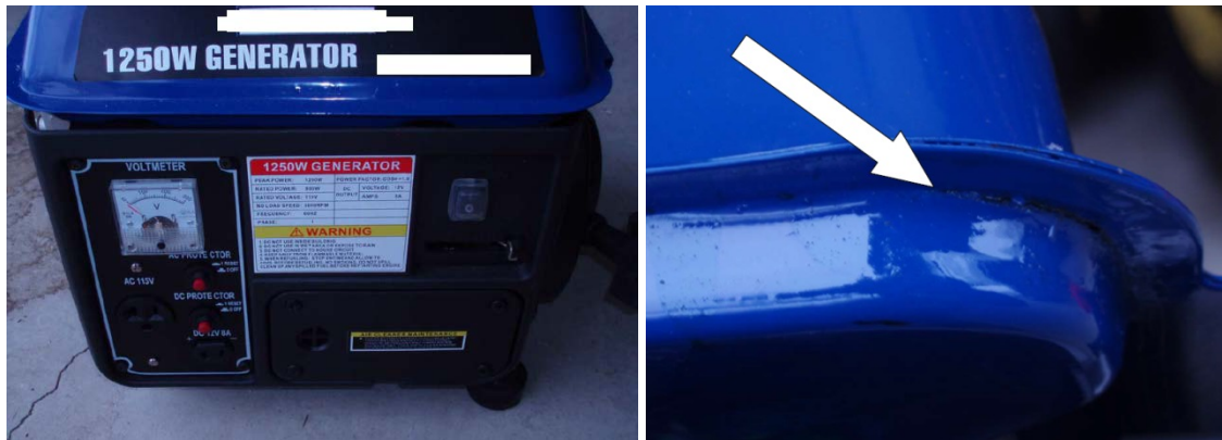
Figure 7 – Subject Portable Generator (Left); Crack in the Fuel Tank Seam, as described by the Complainant (Right)
