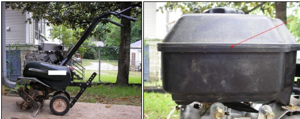
Figure 1 – Subject Tiller (Left); Fuel Tank leaked gasoline at the seam indicated by red arrow as described by complainant (Right)
