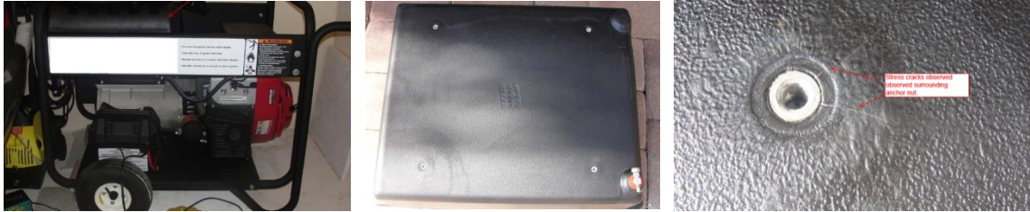
Figure 9 – Subject Portable Generator (Left); Bottom View of the Fuel Tank (Middle); Stress Cracks from an Anchor Nut Indicated by Red Arrows (Right)
