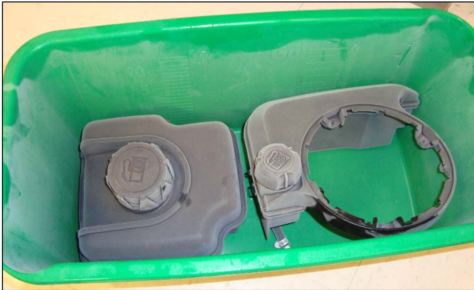
Figure 25 – Brand B and Brand C Tanks after Removing Them from the Cold Chamber
