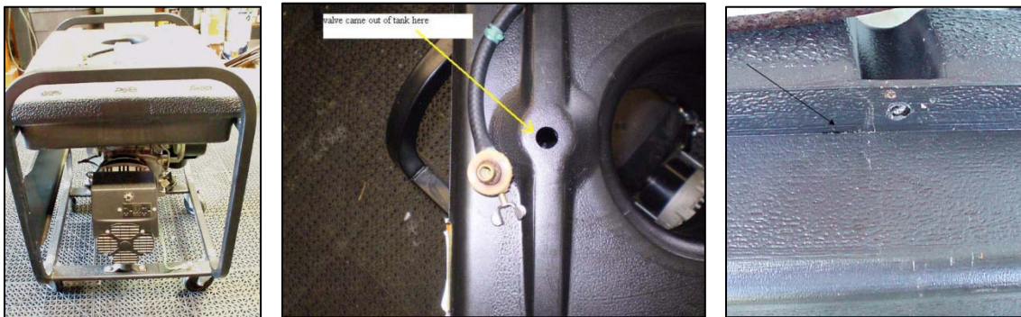
Figure 11 – Subject Portable Generator (Left); Fuel Valve Separated from the Fuel Tank (Middle); and Crack in the Fuel Tank (Right)
