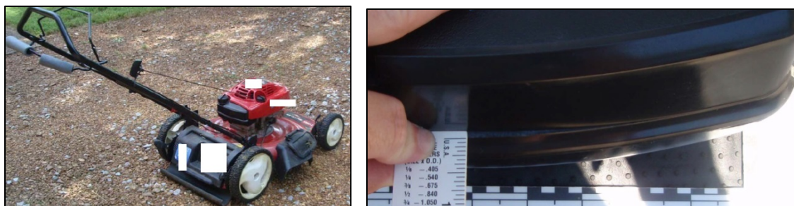
Figure 4 – Subject Mower (Left); Fuel Tank with a Split in the Seam (Right)
