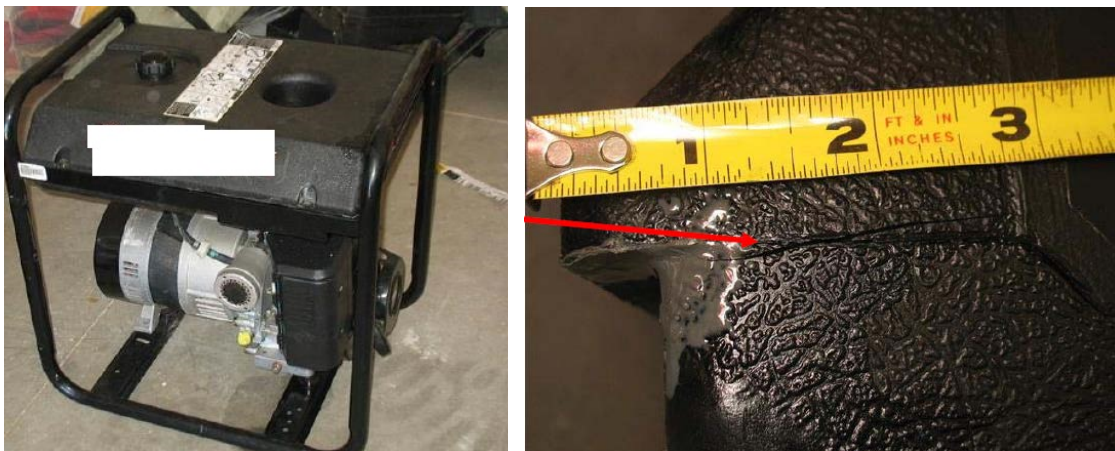
Figure 10 – Subject Portable Generator (Left); Crack in the Fuel Tank where Complainant repaired crack with epoxy (Right)
