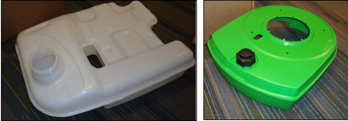
Figure 20 – Brand F Riding Lawn Mower Tank (Left); Brand E Push Lawn Mower Tank (Right)
