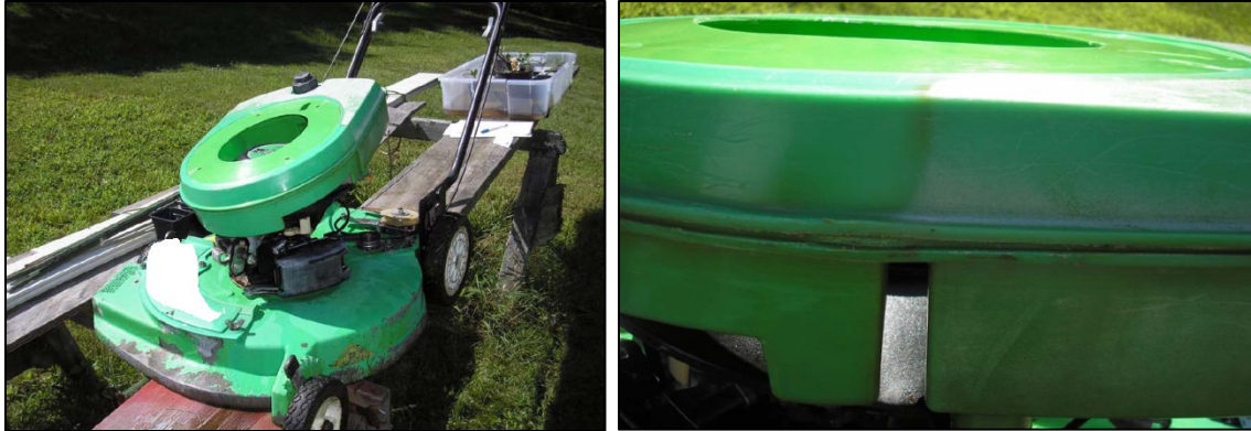
Figure 2 – Subject Push Lawn Mower (Left); Fuel Leaked from the Tank Seam (Right)
