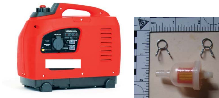
Figure 13 – Subject Portable Generator (Left); Fuel Filter and the Original Hose Clamps/Clips (Right)
