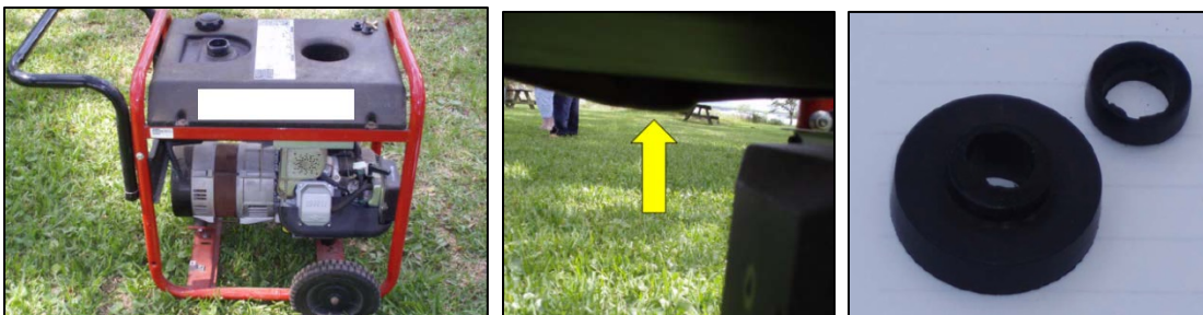
Figure 14 – Subject Generator (Left); Location of Grommet indicated by Yellow Arrow (Middle); Close up of Grommet Deterioration/Failure, which caused Fuel Leak (Right)
