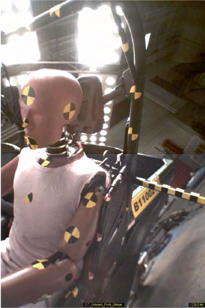
Figure 3.13 Unbelted [redacted] at 60 deg. With Torso Restraint (at time of tether jerk)
