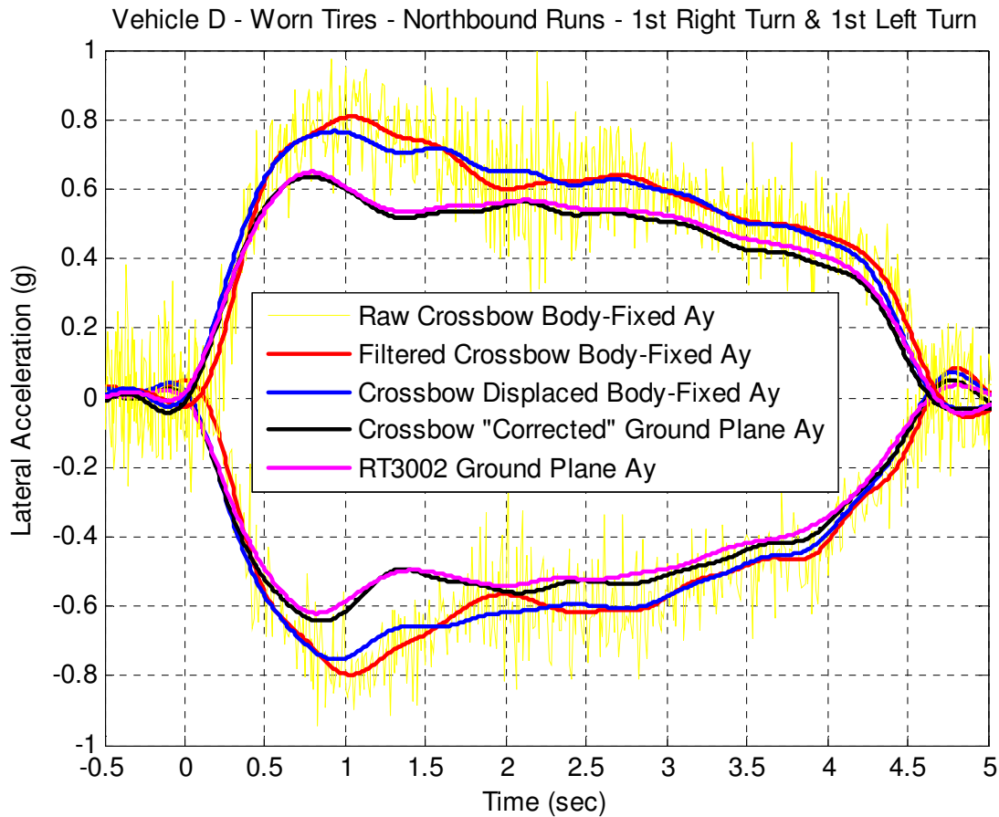
Figure C4: Graphs Showing Various Stages of Calculations Leading to the Method 4 Ground Plane Lateral Acceleration (Along with Method 1 Direct Measurement)
