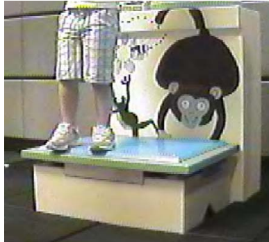
S4-a (CG 17.67 inches, total mass 49.56 lbs, no tip) Figure 21. Session 4, Snapshot of Data Point S4-a
