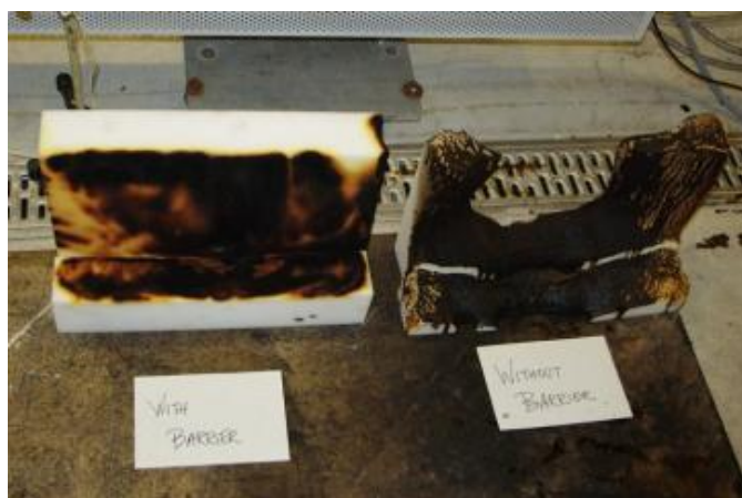
Figure 67. Photo of the comparison between residues of mockups (formulation C1) tested with barrier material (on the left) and without barrier material (on the right).
