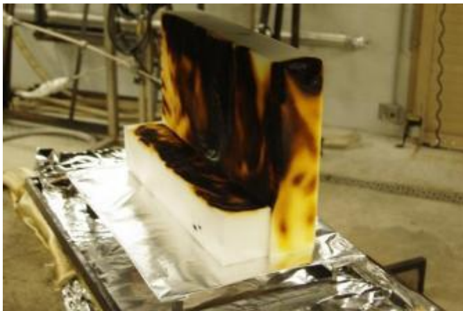
Figure 65. Photo of the residue of the mockup at the end of the test after removing the barrier material, the polyester fabric and the cover fabric.
