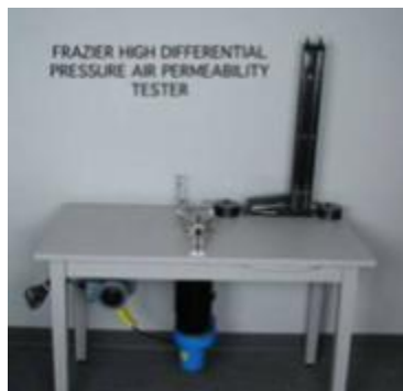
Figure 16. Photograph of the electronic high differential pressure instrument for measuring air permeability.
