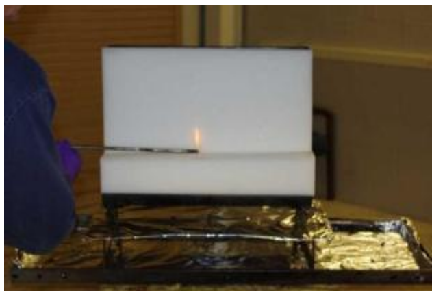
Figure 12. A photo of the 35 mm butane flame impinging for 5 s on a mockup assembly without barrier material in the open-flame test for bare foam.
