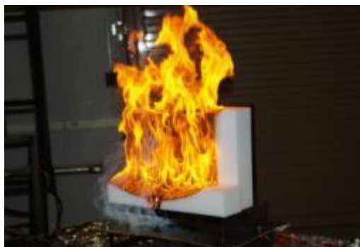
Figure 60. Photo of test with formulation C1 a few seconds before extinguishing the sample. At this stage, flaming liquid material was dripping to the underlying tray, but there was no pool fire (which would sustain flaming and boost the heat release rate through a feedback effect).
