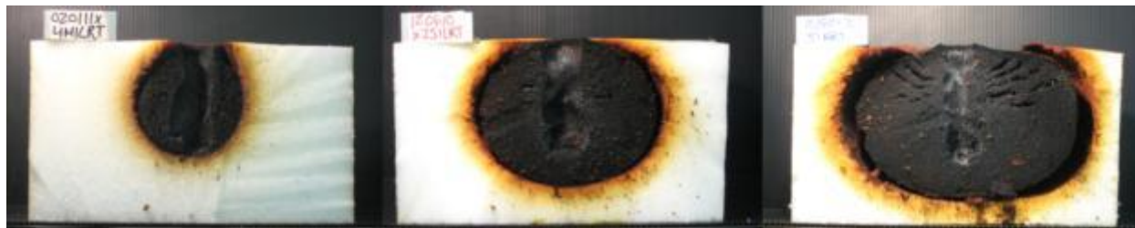
Figure 7. Illustration of the charred material produced in the box test. The respective mass losses were 2 % by mass (left), 4 % by mass (center) and 7 % by mass (right).
