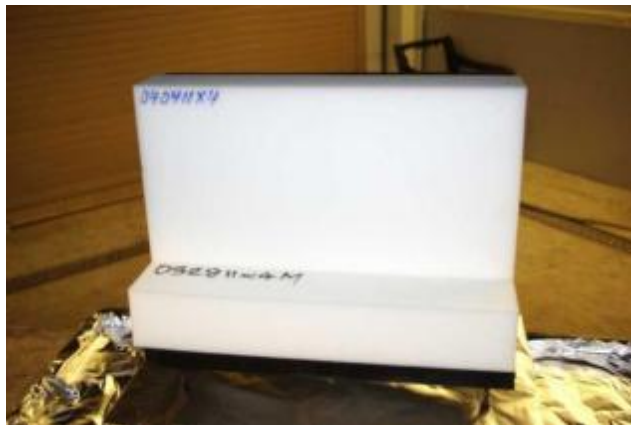
Figure 11. An example of a mockup assembly without a barrier used in the open-flame test for bare foam.
