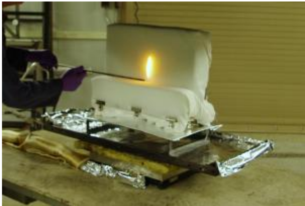
Figure 13. A photo of the 240 mm butane flame impinging for 70 s on the standard polyester fabric covering the foam in the open-flame test with barrier material.
