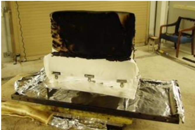
Figure 64. Photo of the residue of the mockup after the open-flame test with barrier material.
