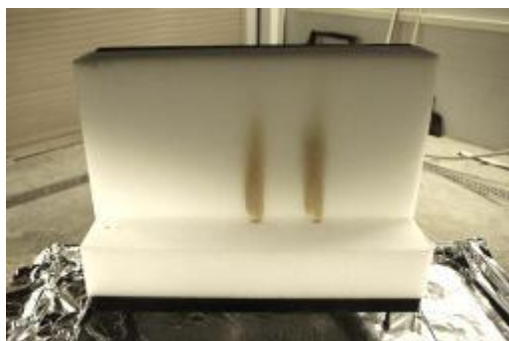
Figure 61. Ignition was not observed after the first 5 s of flame impingement with formulations B5 and C2; a second attempt was carried out by applying the open-flame for another 5 s in a new location 5 inches apart from the original ignition point. Here, a mockup assembly for formulation C2 after attempting ignition twice is shown.
