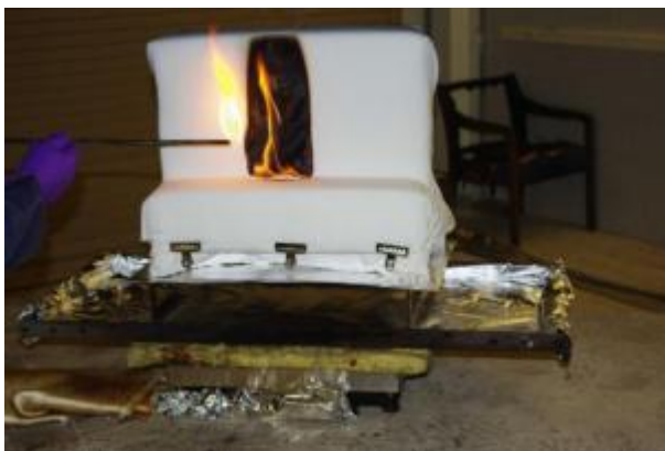
Figure 14. Photo of the open-flame test with barrier material. The 240 mm butane flame was removed from the crevice after 70 s of flame impingement.
