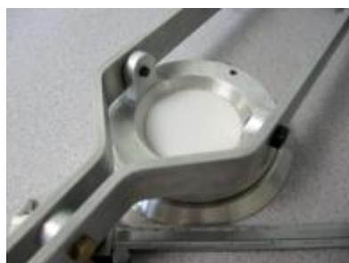
Figure 17. Clamping of the PUF samples during a permeability measurement.
