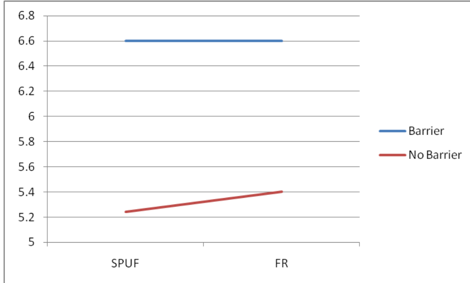
Figure 3. Foam/Fire Barrier Interaction for Time to Peak Heat Release (in Log Seconds)
