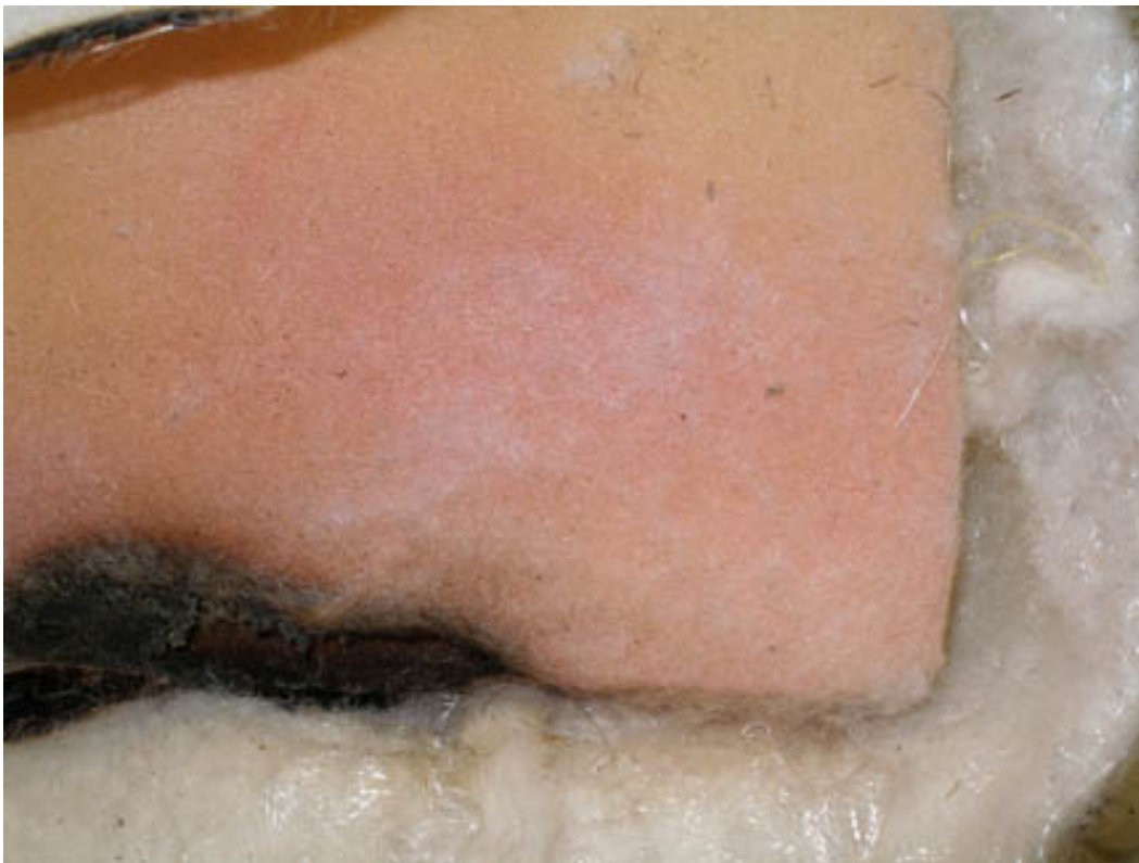
Figure 7. An example of glue (dark pink) and polyester remnants on foam, even though this construction did not call for polyester directly attached to the foam.
