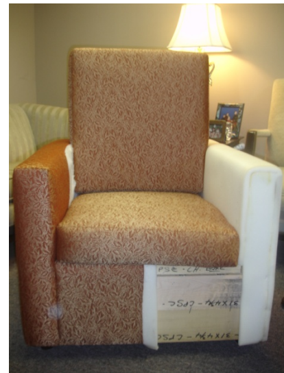
Figure 3. Prototype of Partially Upholstered Chair
