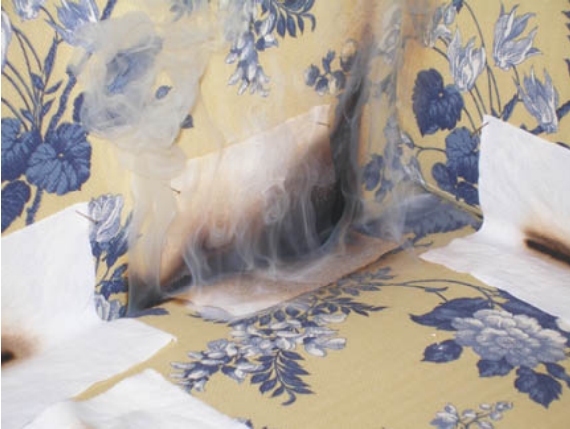
Figure 4. An example of progressive smoldering at the end of the test.
