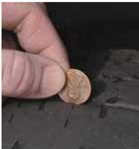
Inadequate Tire Tread
