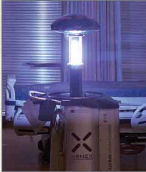
The Xenex germ-busting robot goes to work at the Spinal Cord Injury Center. Milwaukee has two of the robots that obliterate bacteria with 67 pulses of ultraviolet light per second.
