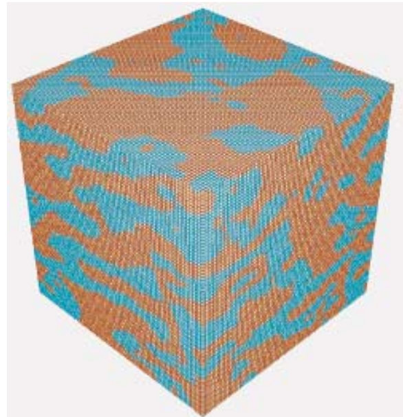
Figure 4: Finite element mesh of a subsection of scaffold shown in Figure 2. The dimension is 274 \mu\text{m} on each side.
