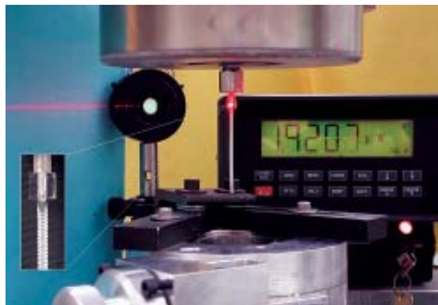
Figure 2: Frustrated Total Internal Reflection optics is installed near the die exit on a capillary rheometer. The amplitude of the reflected light allows a determination of the coating thickness.
